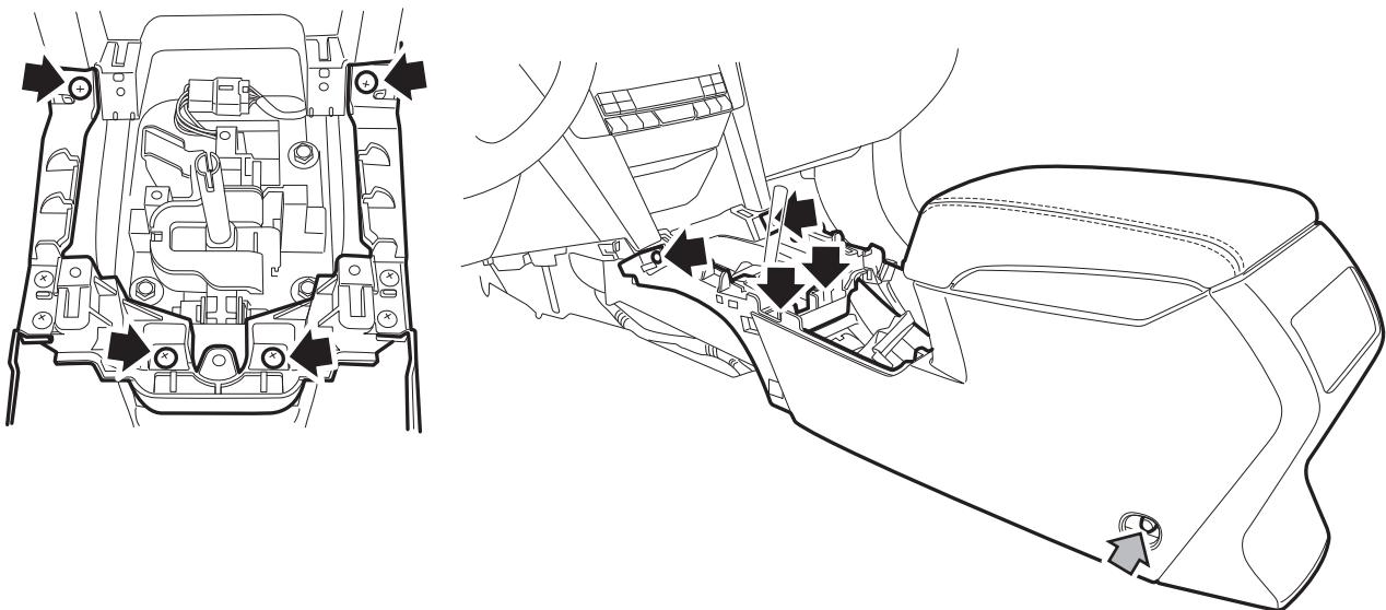
5) Remove the airbag control module.
