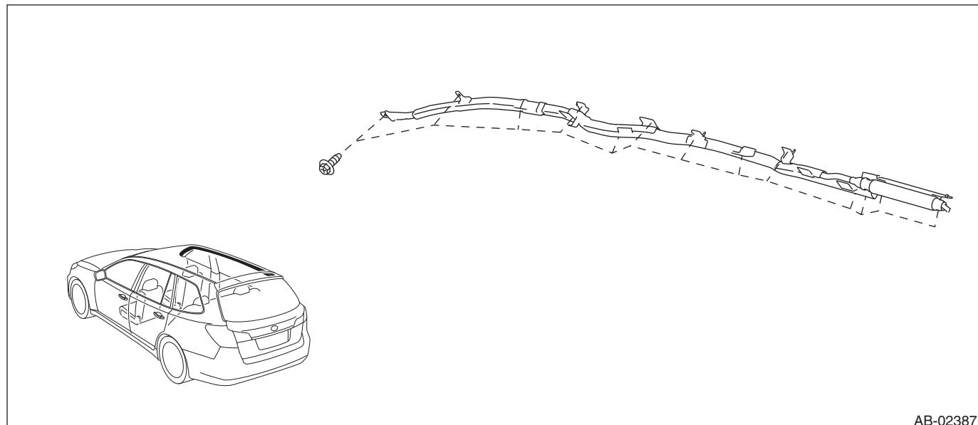
(2) Disconnect the curtain airbag module connector.
