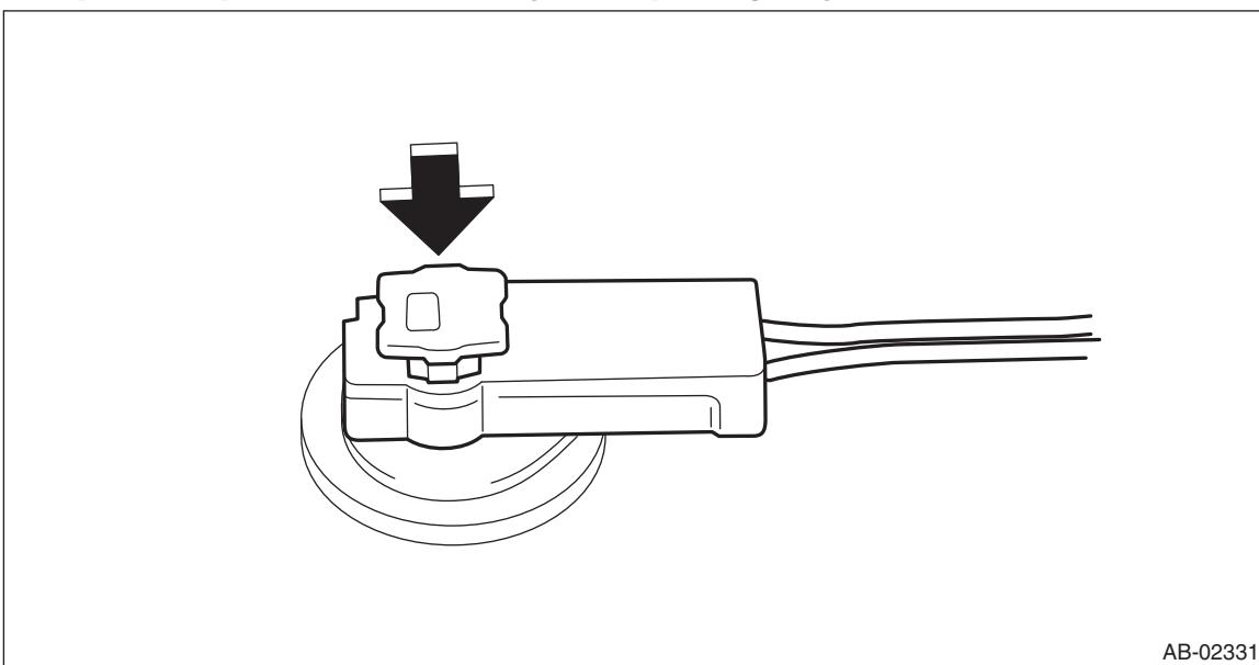
Connect the connector in the reverse order of disconnecting. At this time, be sure to insert it until a clicking sound is heard.
