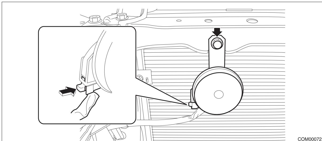
6) Remove the Hi pitch side horn.
