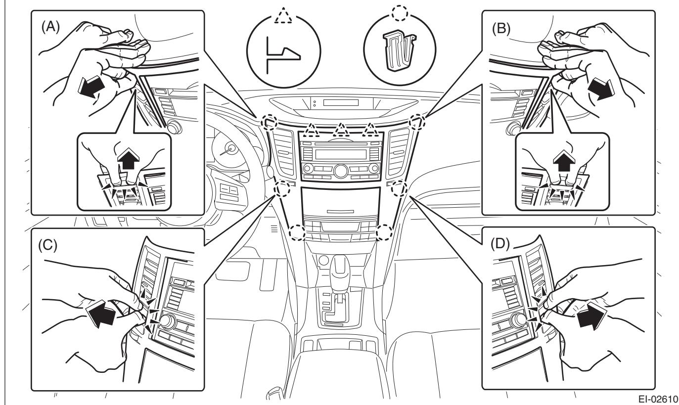
2) Release the claws, and then remove the center grille assembly.
