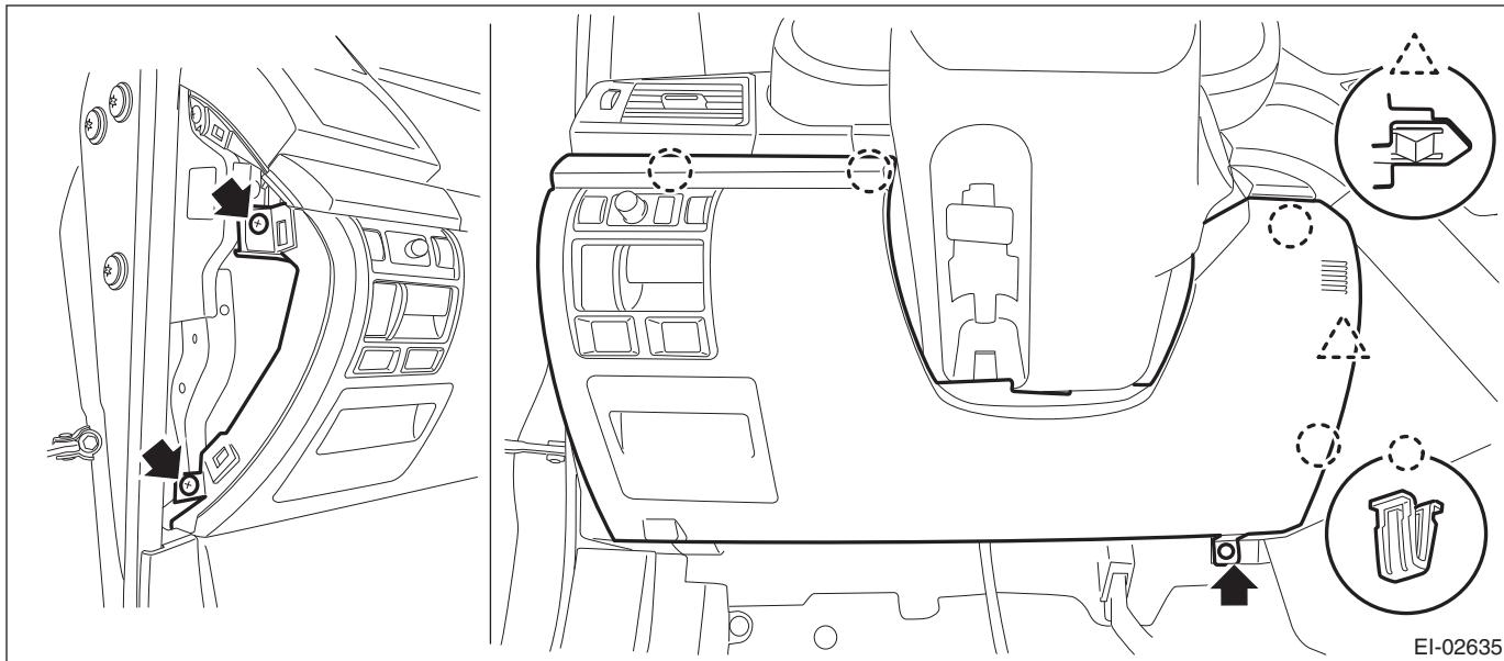
4) Remove the screw and remove the in-vehicle sensor from the instrument lower cover.
