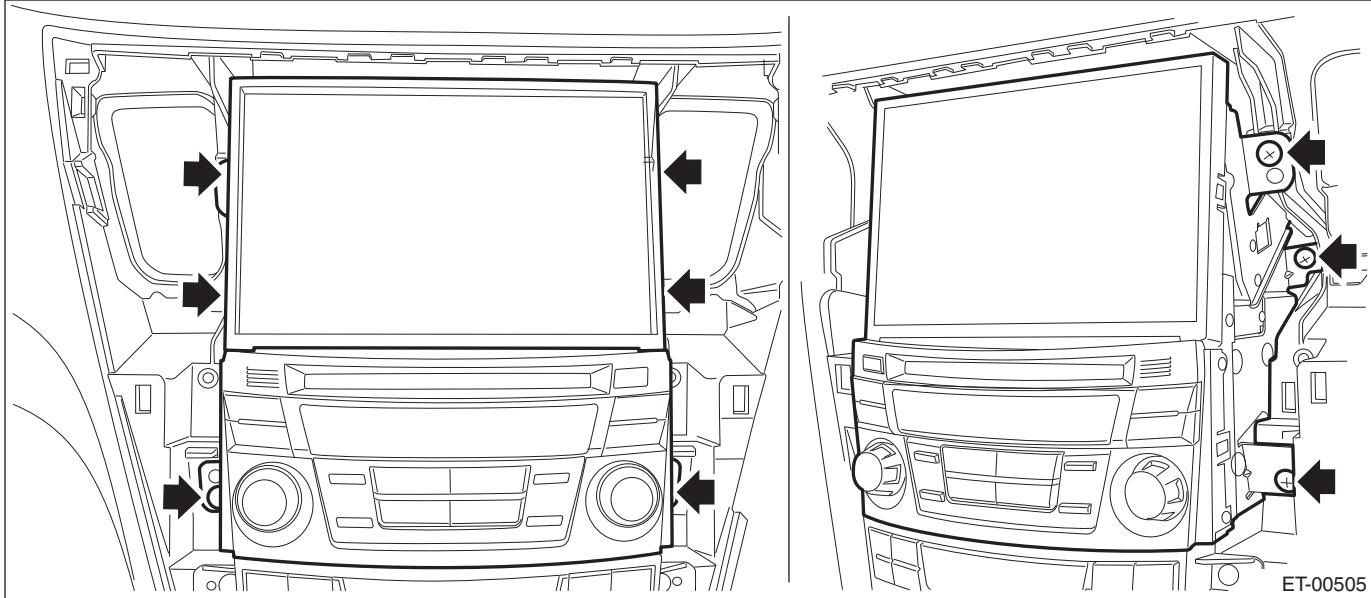
5) Remove the control panel.
