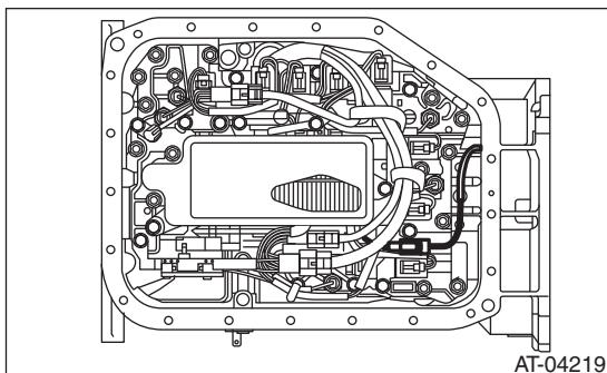
3) Apply proper amount of liquid gasket to the entire oil pan mating surface.
