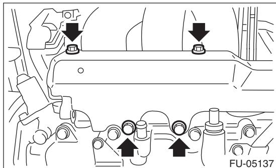
(11) Remove the ignition coil. <Ref. to IG(H6DO)-7, REMOVAL, Ignition Coil.>
