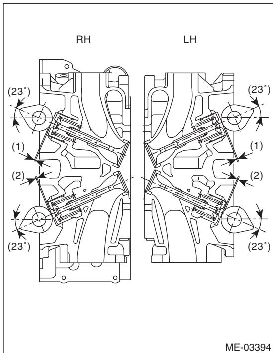
(1) Valve clearance (Intake side)
