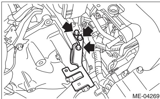
11) Install the engine harness connector to the engine hanger bracket.
