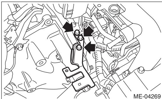
14) Remove the throttle body from the intake manifold.
