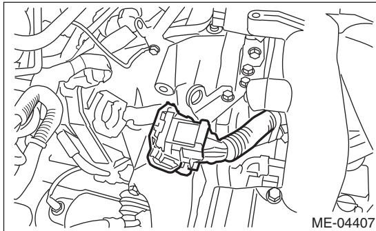
12) Connect the connector to the throttle body.
