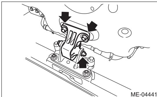
18) Remove the front mounting bracket from the cradle.
