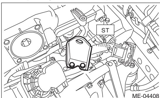
16) Support the engine with a lifting device and wire ropes.
