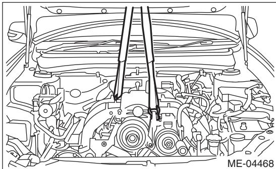
4) Install the radiator main fan & fan motor and radiator sub fan & fan motor. <Ref. to CO(H6DO)-22, INSTALLATION, Radiator Main Fan and Fan Motor.> <Ref. to CO(H6DO)-24, INSTALLATION, Radiator Sub Fan and Fan Motor.>
