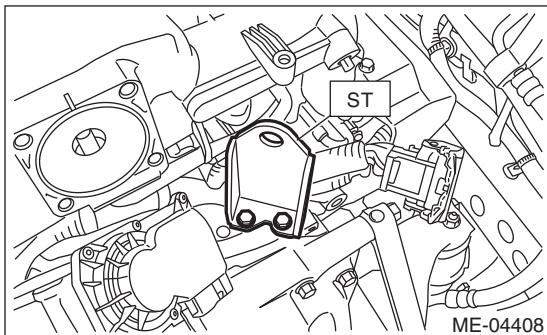
9) Install the throttle body to intake manifold.
