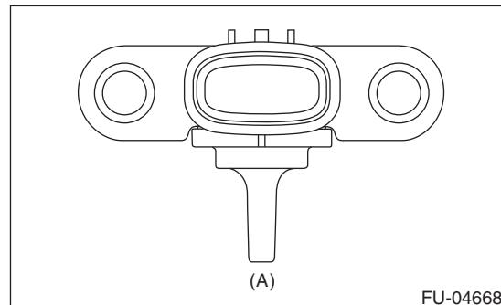
4) Check the voltage when generating vacuum and positive pressure using Mighty Vac.
