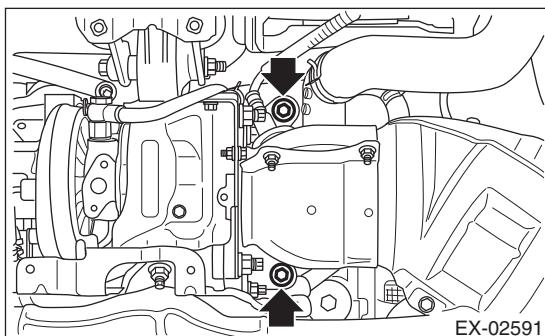
3) Set the oil catch tank to the turbocharger, and attach the bolt and nut which secure the oil catch tank to the turbocharger and oil catch tank stay.
