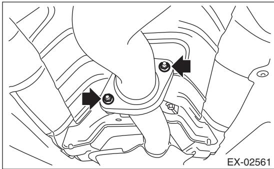
7) Assemble the center exhaust pipe (rear) to the center exhaust pipe (front).
