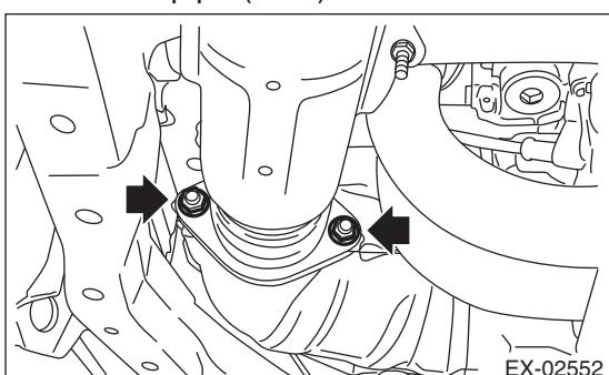
16) Remove the rear exhaust pipe from the center exhaust pipe (rear).
