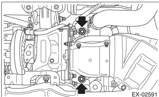
21) While holding the front exhaust pipe with transmission jack, remove the nuts which hold the front exhaust pipe to the cylinder head exhaust port, and remove the front exhaust pipe.
