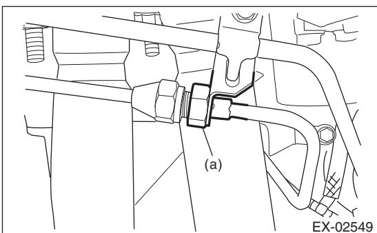
**Tightening torque:****T1: 6.4 N·m (0.7 kgf·m, 4.7 ft-lb)****T2: 20 N·m (2.0 kgf·m, 14.8 ft-lb)**
