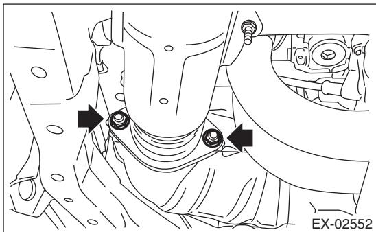
8) Tighten the bolts which hold center exhaust pipe (rear) to the hanger bracket.
