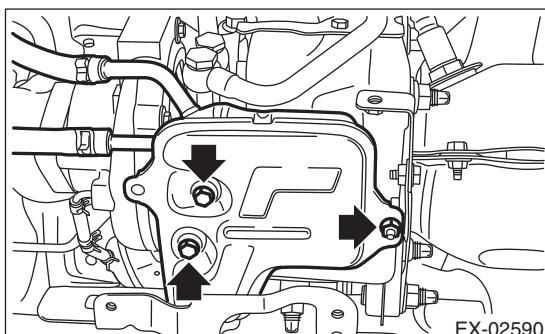
20) Remove the bolts which secure the turbocharger stay.
