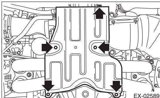
19) Remove bolts and nuts which secure the oil catch tank to the turbocharger and oil catch tank stay, and remove the oil catch tank from the turbocharger.
