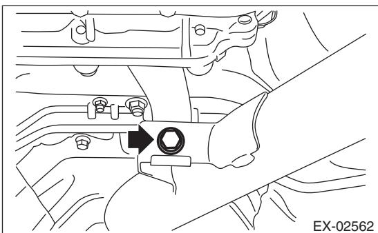
9) Install the bolts which secure the intake duct to the turbocharger, and connect the air control hose (A).
