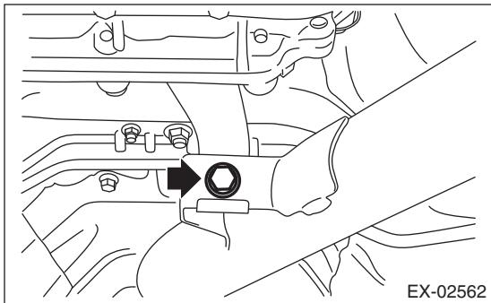
6) Install the rear exhaust pipe to the center exhaust pipe (rear).
