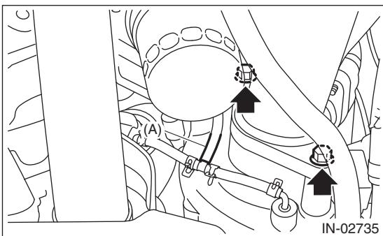
10) Install the bolt which holds oil inlet pipe C (C) and oil inlet pipe A (A), and install oil inlet pipe B (B) to oil inlet pipe A (A).
