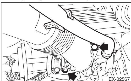
14) Install the radiator sub fan motor assembly. <Ref. to CO(H4DOTC)-27, INSTALLATION, Radiator Sub Fan and Fan Motor.>
