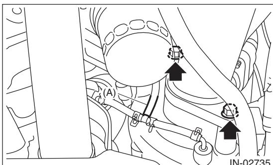
15) Remove the center exhaust pipe (rear) from the center exhaust pipe (front).
