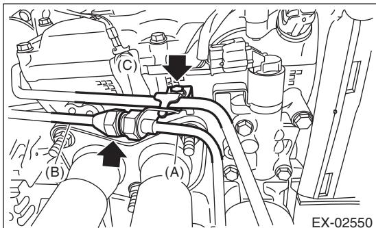
14) Disconnect the air control hose (A), and loosen the bolts which secure the intake duct to the turbocharger.
