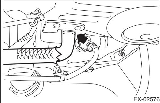
16) Connect connectors to the front oxygen (A/F) sensor and rear oxygen sensor, and secure the front oxygen (A/F) sensor harness and rear oxygen sensor harness with the clip (A).
