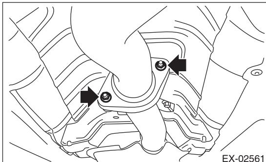
17) Remove the bolt which holds center exhaust pipe (rear) to the hanger bracket, and remove the center exhaust pipe (rear).
