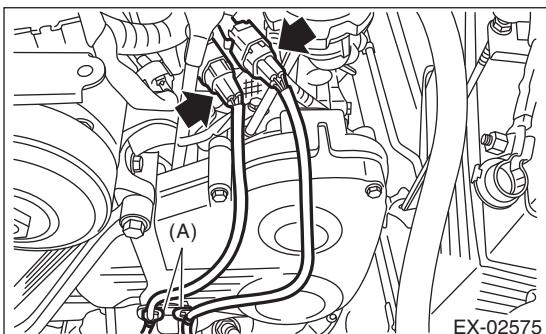
9) Disconnect the engine coolant hose from the water tank pipe and water pump.
