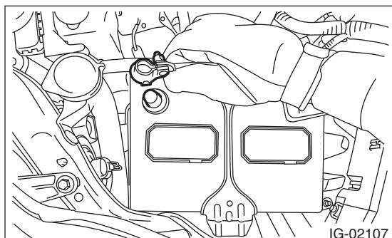
4) Remove the intercooler. <Ref. to IN(H4DOTC)-17, REMOVAL, Intercooler.>
