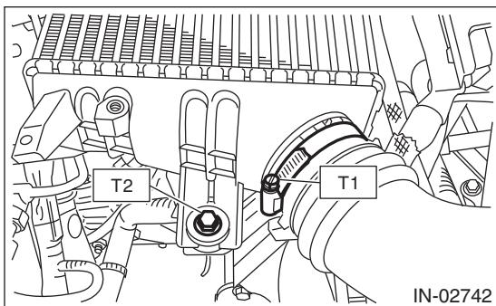
10) Install the bolts which secure the intercooler to the intercooler stay LH, and tighten the clamp which holds the intake duct to the intercooler.
