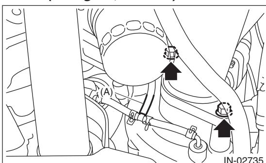
2) Install the air by-pass valve and air intake boot to the intake duct, and connect the vacuum hose to the intake duct.
