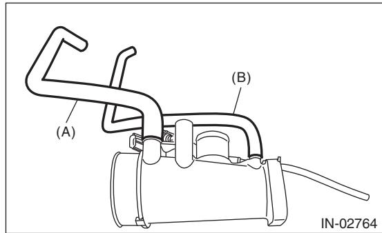
2) Remove the wastegate control solenoid valve and air control hose from the intake duct.
