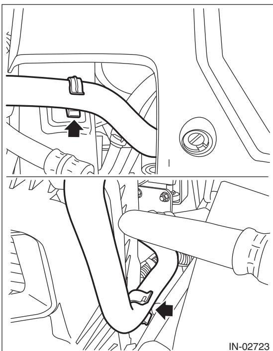
4) Disconnect the connector (A) from the mass air flow and intake air temperature sensor, and remove the clip (B) which holds the mass air flow and intake air temperature sensor harness.
