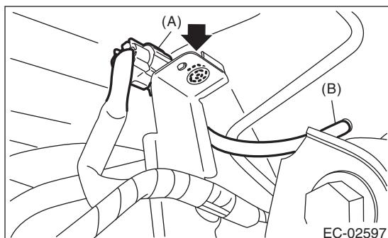
7) Disconnect the pressure hose from fuel tank pressure sensor and remove the fuel tank pressure sensor.
