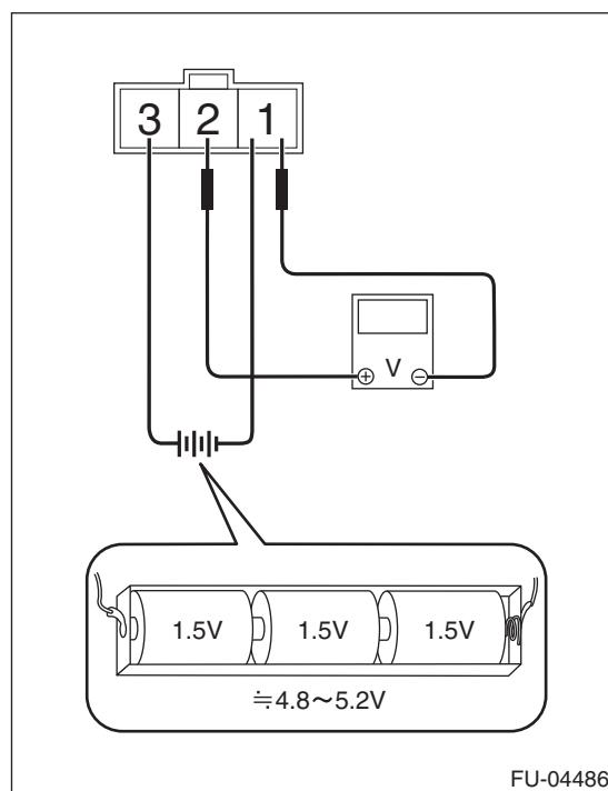
3) Check the voltage at a normal atmospheric pressure.
