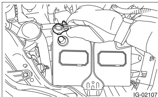
2) Open the fuel filler lid and remove the fuel filler cap.
