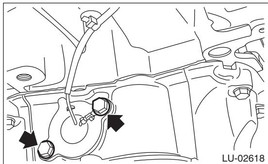
2) Hold the oil level switch harness with clip.
