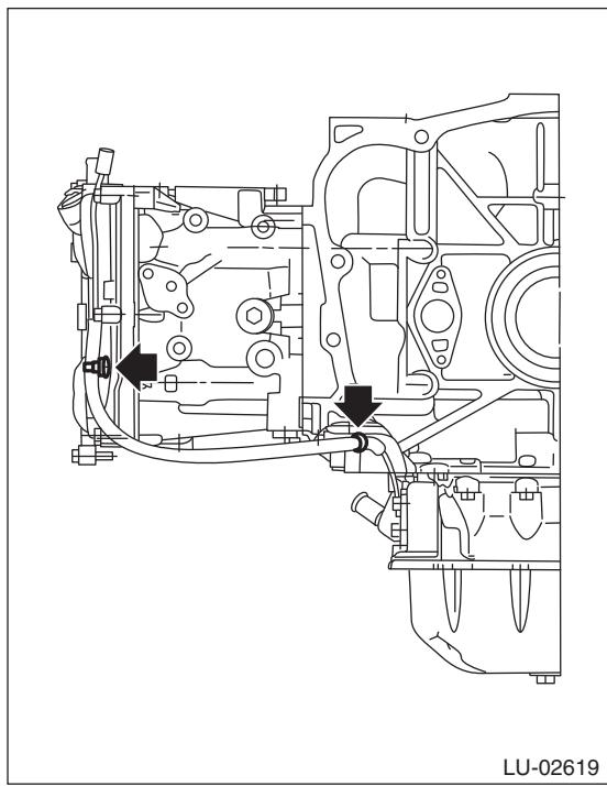
3) Connect the connector of oil level switch to the engine harness.
