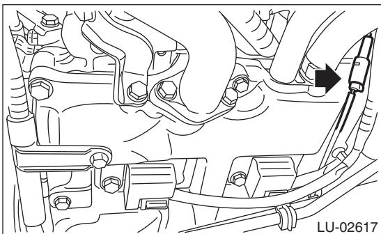
6) Remove the clip holding the oil level switch harness.
