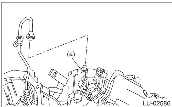
13) Remove the bolt (B) which secures the oil inlet pipe B (A) to the cylinder head and the stay to remove the oil inlet pipe B (A).
