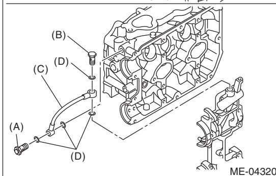
(A) Union bolt with filter (with protrusion)
