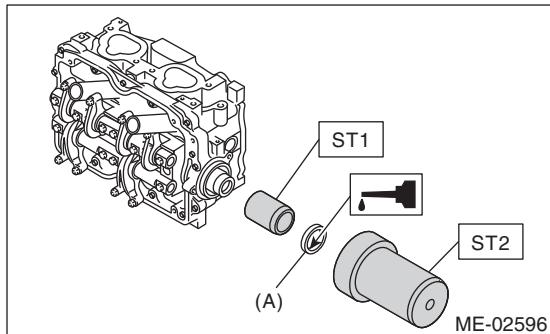
4) Apply a coat of engine oil to plug periphery and install the plug (A) using ST.
