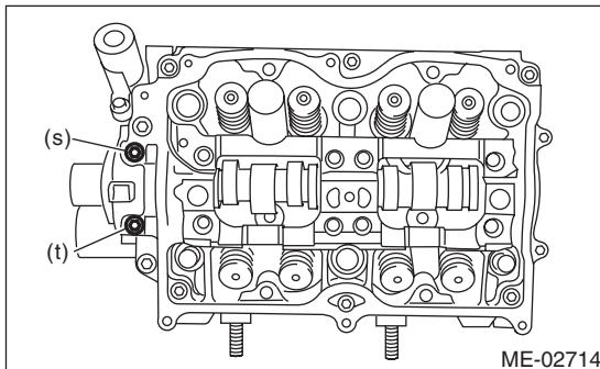
(3) Apply a coat of engine oil to camshaft oil seal periphery and oil seal lips and install the oil seal (A) on camshaft using ST1 and ST2.
