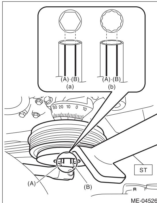
(a) When using 6-point socket
