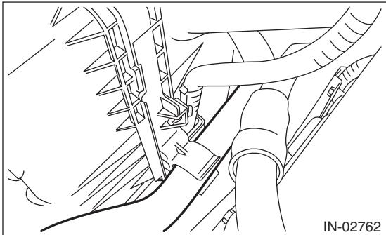
4) Disconnect the connector (A) from the mass air flow and intake air temperature sensor, and remove the clip (B).
