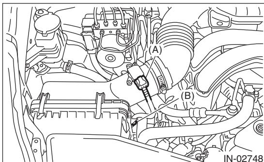
5) Connect the power steering oil pressure hose (suction hose) to the clip on the side of air cleaner case (rear).
