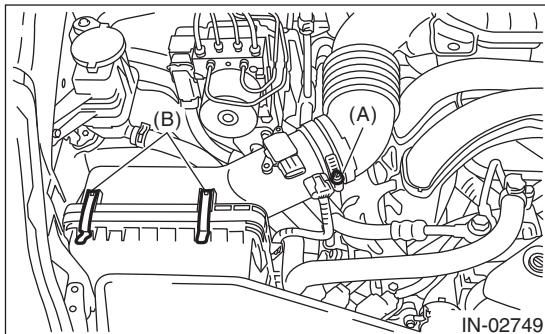
7) Remove the air cleaner case (rear) and air cleaner element.
