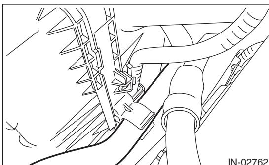
6) Install the air intake duct. <Ref. to IN(H4SO)-9, INSTALLATION, Air Intake Duct.>
