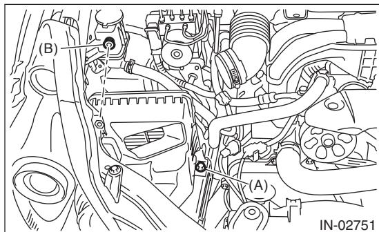
2) Install the air cleaner case (rear) and the air cleaner element.
