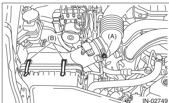
4) Connect the connector (A) to the mass air flow and intake air temperature sensor and secure the harness with clip (B).
