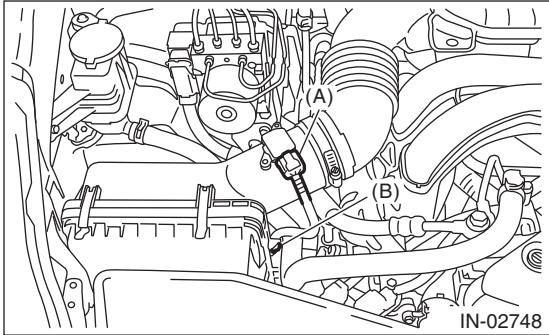
5) Loosen the clamp (A) which connects the air cleaner case and air intake boot assembly.
