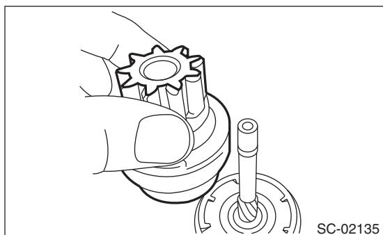
(3) Install stopper (B) to the shaft, then install snap ring (A).
