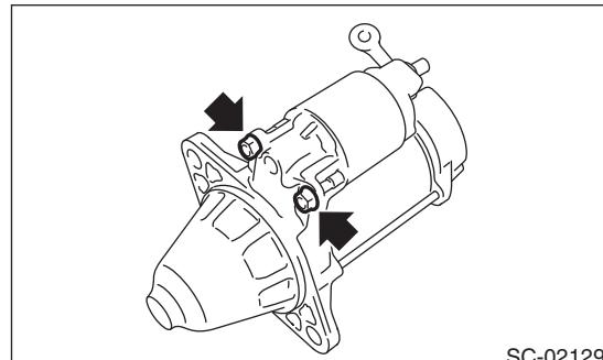
12) Install the harness to the terminal M (A) of the magnet switch assembly, and tighten the nut.
