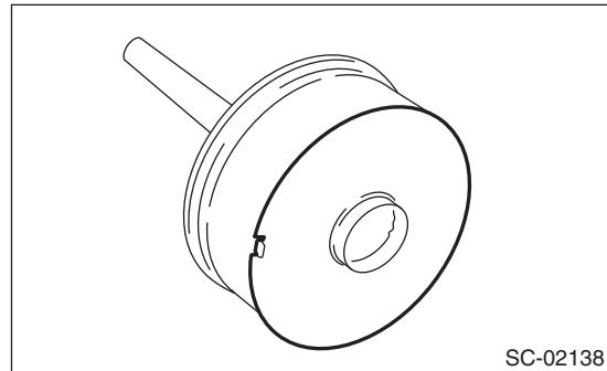
(2) Remove the planetary gear.
