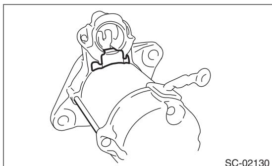
11) Install the magnet switch assembly to the starter housing, and tighten the nuts.
