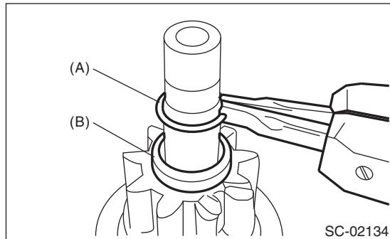
(4) Using a press, pressure fit stopper (B) into snap ring (A).
