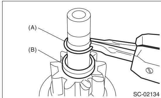
(3) Remove the overrunning clutch from the shaft.
