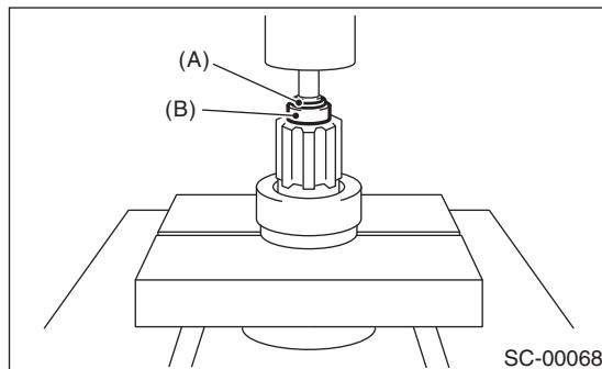
7) Assemble the overrunning clutch, shock absorber, and shaft to the yoke as a single unit
