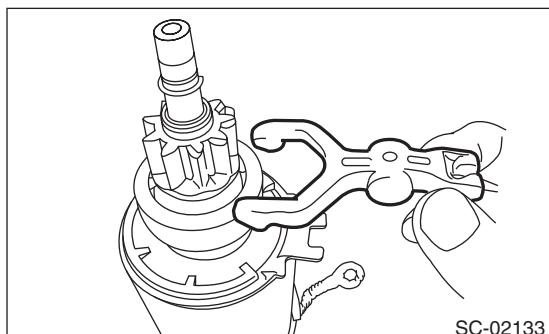
9) Install the starter housing, and tighten through bolts on both sides.
