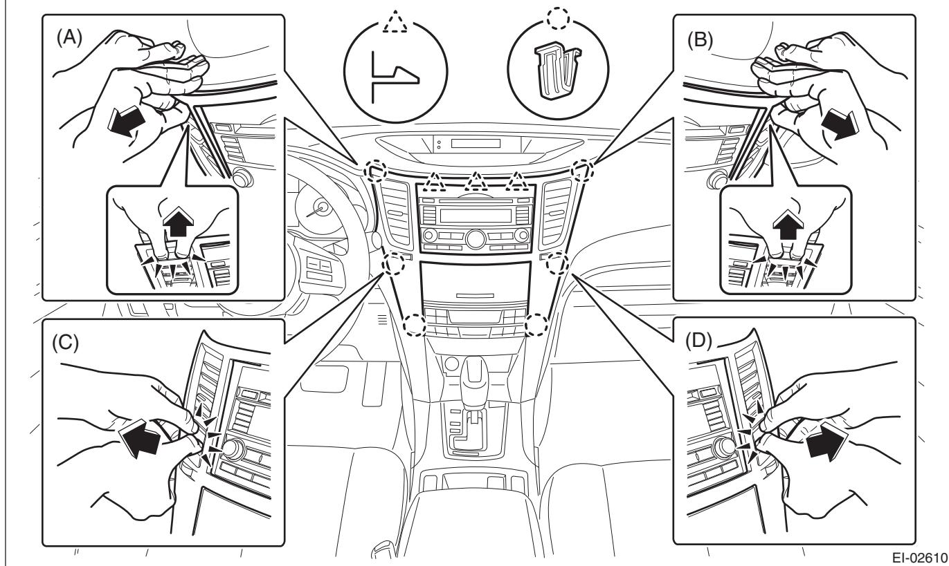
3) Remove the screw and release the claws, then detach the starter cover assembly.
