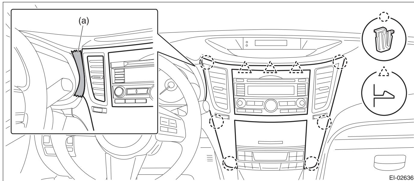
(2) Insert a finger into the air vent grille and release the left and right clips at the top of the center panel.
