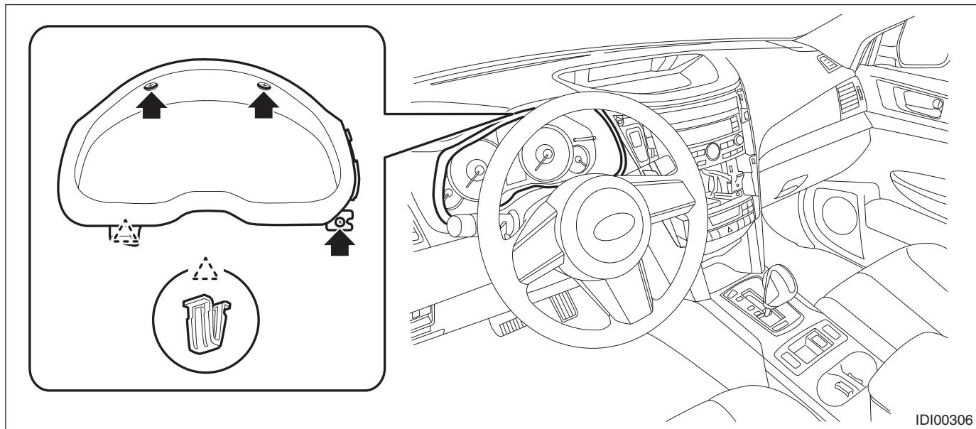
6) Remove the combination meter assembly.
