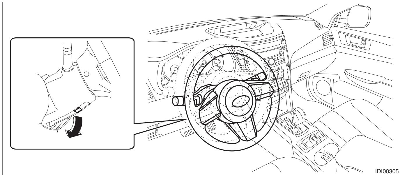
5) Release the screws and clips, then detach the meter visor assembly.
