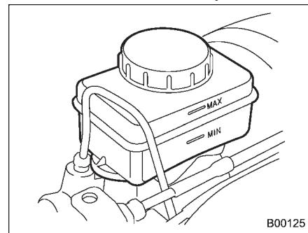
Check the fluid level on the outside of the reservoir. If the level is below "MIN", add the recommended brake fluid to "MAX".
