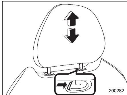
To raise the head restraint, pull it up. To lower it, push the head restraint down while pressing the release button on the
