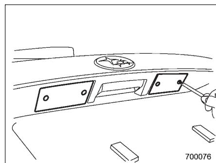
1. Remove the mounting screws using a Phillips screwdriver.
