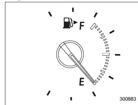
The rim of the fuel gauge flashes five times when the amount of remaining fuel reaches 2.6 US gal (10 liters, 2.2 Imp gal). If you turn the ignition switch to the "LOCK" position and back to the "ON" position, the rim will again flash five times.
