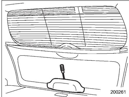
1. Remove the access cover at the bottom-center of the rear gate trim using flat-head screwdriver.
