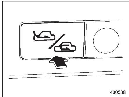
Select air flow by pushing the air inlet selection button “ ”. The selected air inlet setting is shown on the control panel.
