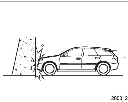
A head-on collision against a thick concrete wall at a vehicle speed of 12 to 19 mph (20 to 30 km/h) or higher activates only the driver's SRS frontal airbag or both driver's and front passenger's SRS frontal airbags. The airbag(s) will also be activated when the vehicle is exposed to a frontal impact similar in fashion and magnitude to the collision described above.
