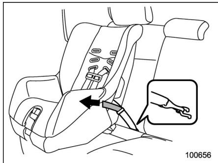
2. If your child restraint system is of a flexible attachment type (which uses tether belts to connect the child restraint system properly to the lower anchorages), while pushing the child restraint into the seat cushion, pull both left and right lower tether belts up to secure the child restraint system firmly by taking up the slack in the belt.
