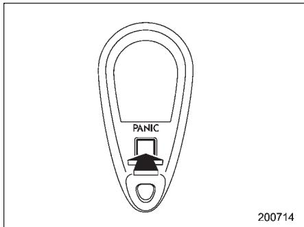
A “PANIC” button is located on the back of the transmitter.
