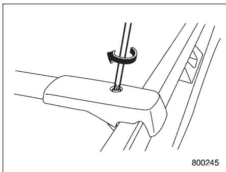
6. Adjust the alignment of the crossbar on the roof rails, and if available, use a T-30 torx® bit and torque wrench and tighten the T-30 torx® head screws to 30 to 35 lbf-in (3.4 to 4.0 N·m, 0.35 to 0.41 kgf·m) of torque (or tighten securely with the torx® wrench provided).
