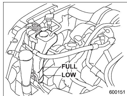
6. Pour the coolant and fill to the reservoir tank's "FULL" level mark.
