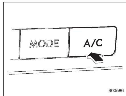
If the windshield starts to fog when the climate control system is operated in the AUTO mode, push the air conditioner button "A/C" to defog and dehumidify.
