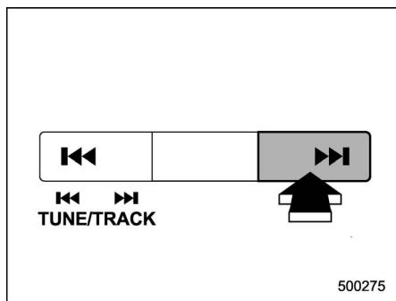
Press the "▶" side of the TUNE/TRACK button continuously to fast-forward the disc/folder.
