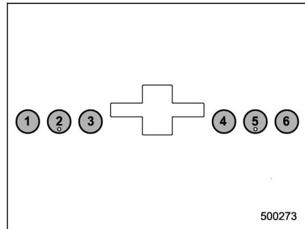
Presetting a station with a preset button allows you to select that station in a single operation. Up to six AM, FM1 and FM2 stations each may be preset.
