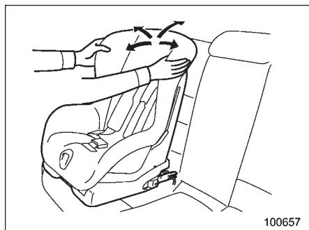
4. Before seating a child in the child restraint system, try to move seat back and forth and left and right to verify that it is held securely in position.
