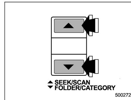
Press the "▲" side of the SEEK/SCAN button to change the radio to the SCAN mode. In this mode, the radio scans through the channel until a station is found. The radio will stop at the station for five seconds while displaying the channel number, after which scanning will continue until the entire channel has been scanned from the low end to the high end. Press the "▲" side of the button again to cancel the SCAN mode and to stop on any displayed channel.
