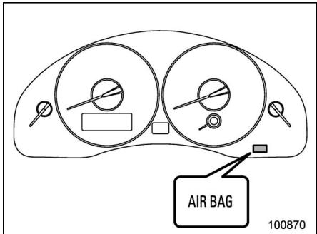
SRS airbag system warning light (Turbo models)
