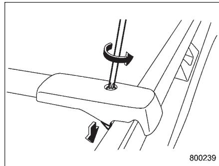
1. Loosen and remove the T-30 torx® head screw from the top of each crossbar end support.
