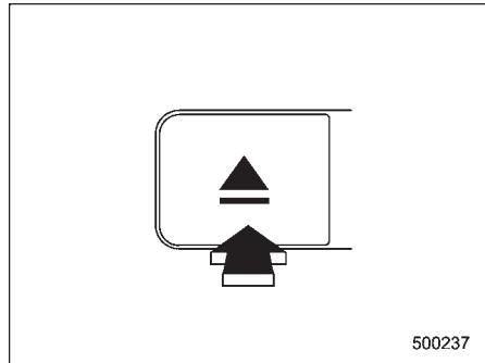
1. If you continue to press the "▲" button, the player will produce beep sound and will enter the all disc ejection mode. At this time, the disc number indicator and "ALL EJECT" indicator will flash.
