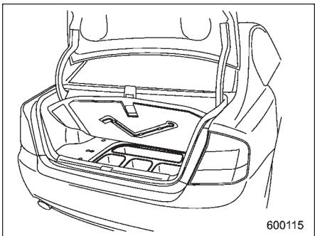
2. Remove the jack handle from the back of the floor cover.
