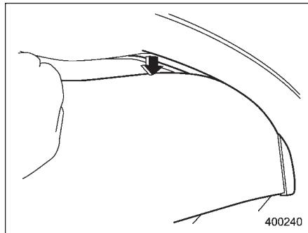
the rear gate board, rotate the rear gate board toward you, and pull it out downward.
