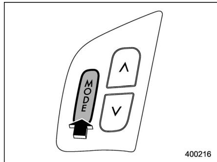
This button is used to select the desired audio mode. Each time it is pressed, the mode changes to the next one in the following sequence:
