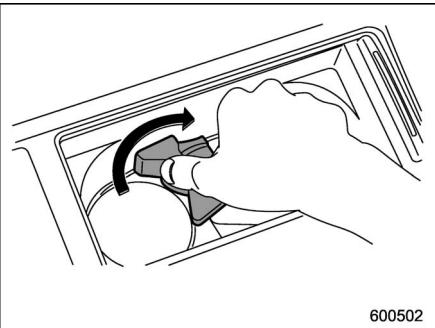
Insert the protrusion on the back of the divider plate into the hole in the center of the console box. Grasp the divider plate at the base, and turn it clockwise to fit it.
