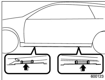
8. Place the jack under the side sill at the front or rear jack-up point closest to the flat tire.
