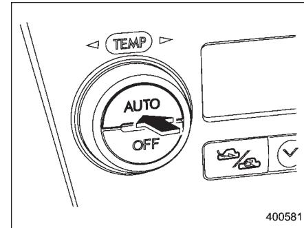
When the "AUTO" button is pressed, the indicator light "AUTO" on the display comes on. In this state, fan speed, air flow distribution, air-inlet control, and air conditioner compressor operation are automatically controlled.
