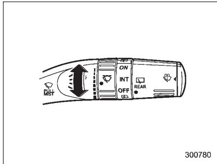
When the wiper switch is in the
