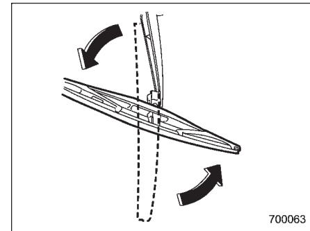
2. Turn the wiper blade assembly counterclockwise.
