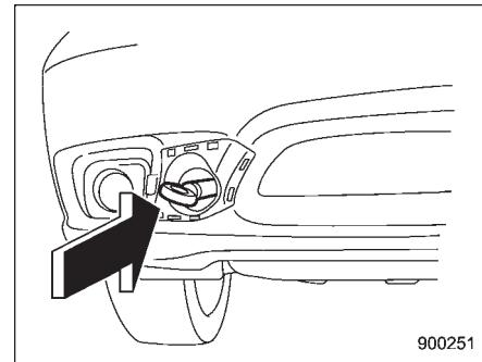
5. Screw the towing hook into the thread hole until the threads can no longer be seen.
