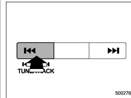
Press the "◀" side of the TUNE/TRACK button continuously to fast-reverse the disc/folder.
