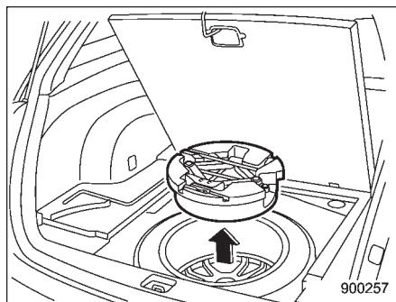
**Station wagon:** To take out the jack and maintenance tools, open the center lid and remove the bucket from the center of the spare tire. Then, take the jack out of the bucket.
