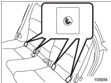
You will find marks “
