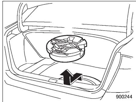
**Sedan:** To take out the jack and maintenance tools, open the floor cover and remove the bucket from the center of the spare tire. Then, take the jack out of the bucket.
