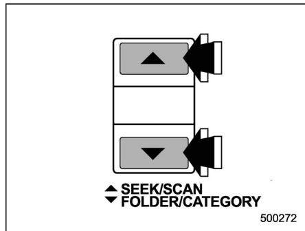
If you press the "▲" or "▼" side of the SEEK/SCAN button briefly, the radio will automatically search for a receivable station and stop at the first one it finds. This function may not be available, however, when radio signals are weak. In such a situation, perform manual tuning to
