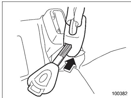
1. Insert a key or other hard pointed object into the slot in the connector (buckle) on the right-hand side and push it in, and the connector (tongue) plate will disconnect from the buckle.
