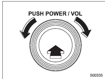
The dial is used for both power (ON/OFF) and volume control. The radio is turned ON and OFF by pushing the dial and the volume is controlled by turning the dial. The dial can also be used for tone and balance adjustment.
