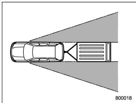
After hitching a trailer to your vehicle, check that the standard side mirrors provide a good rearward field of view without significant blind spots. If significant blind spots occur with the vehicle's standard side mirrors, use towing mirrors that conform with Federal, state/province and/or other applicable regulations.
