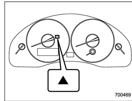
When Intelligent (I) mode is selected in vehicles equipped with a manual transmission, a shift-up indicator "▲" in the tachometer will blink to signal the best time to shift gears for maximum fuel efficiency.
