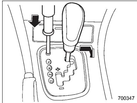
4. Insert the screwdriver into the hole.
