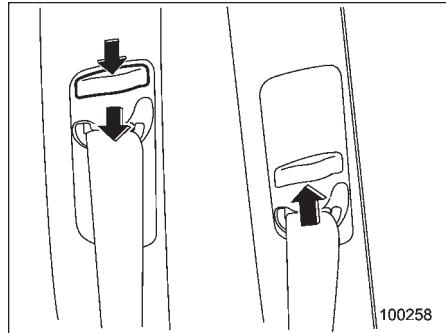
The shoulder belt anchor height should be adjusted to the position best suited for the driver/front passenger. To lower the anchor height, push the release button and slide the anchor down. To raise the anchor height, slide the anchor up. Pull down on the anchor to make sure that it is locked in place.
