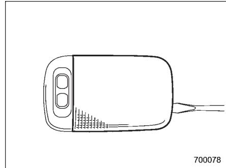
1. Remove the cargo area light assembly by prying the edge of the light with a flat-head screwdriver.
