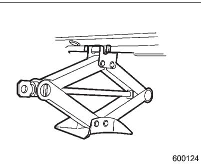
Turn the jackscrew by hand until the jack head engages firmly into the jack-up point.
