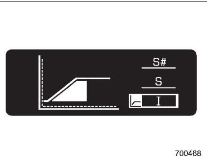
The Intelligent (I) mode provides well-balanced performance with greater fuel efficiency and smooth driveability without stress. Power delivery is moderate during acceleration for maximum fuel efficiency. This is ideal for around-town driving and situations that do not require full power output. It provides better control in difficult driving conditions, such as slippery roads or loose surfaces, due to gentler throttle response.
