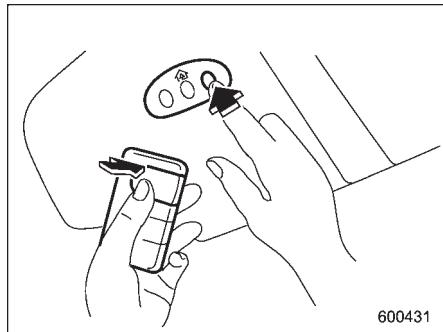
4. Using both hands, simultaneously push the hand-held transmitter button and the desired HomeLink® button. DO NOT release the buttons until step 5 has been completed.
