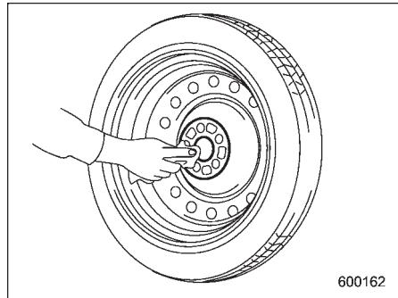
11. Before putting the spare tire on, clean the mounting surface of the wheel and hub with a cloth.
