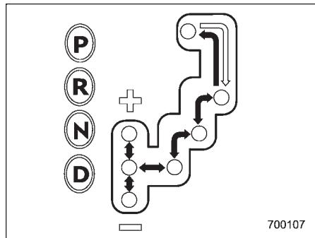
□: Shift possible with brake pedal depressed
