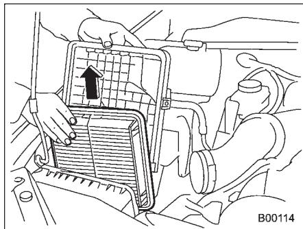
5. Open the air cleaner case cover and remove the air cleaner element.
