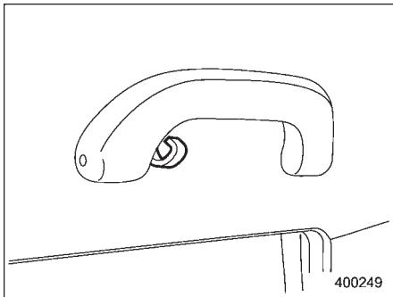
The coat hook is attached to each rear passenger's hand grip.
