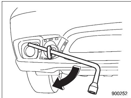
6. Tighten the towing hook securely using a wheel nut wrench.
