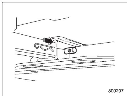
3. Insert the safety pin into the hitch pin securely.
