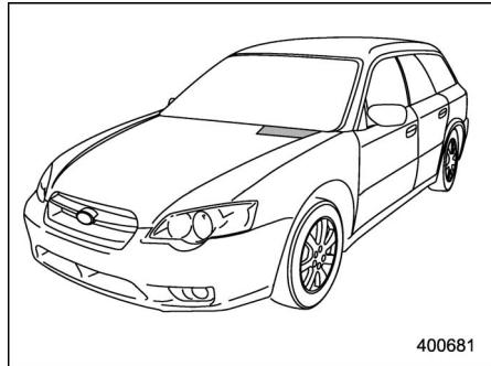
Always keep the front ventilator inlet grille free of snow, leaves, or other obstructions to ensure efficient heating and defrosting. Since the condenser is located in front of the radiator, this area should be kept clean because cooling performance is impaired by any accumulation of insects and leaves on the condenser.
