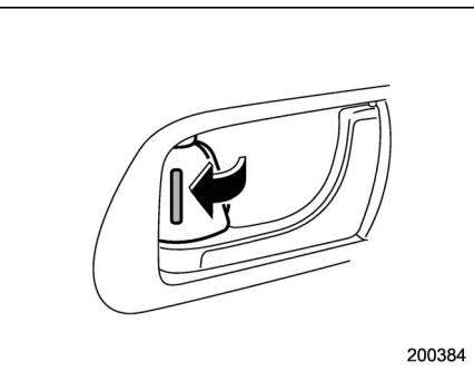
To lock the door from the inside, rotate the lock lever rearward.
