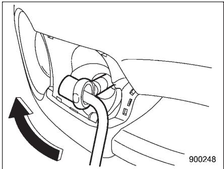
5. Tighten the towing hook securely using a wheel nut wrench.
