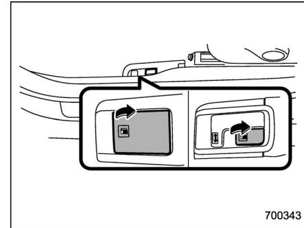
1. To open the fuel filler lid, pull the lid release lever. The lever is on the floor at the left of the driver's seat.
