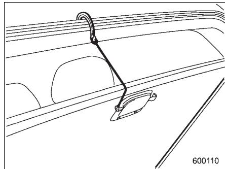
2. To keep the lid open, hang the hook (provided on the back of the lid) on the rear edge of the roof.
