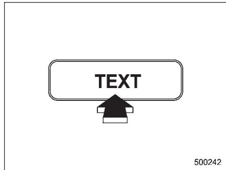
If you press the "TEXT" button for 0.5 second or longer during playback of an MP3/WMA file, the indication will change to the next one in the following sequence.
