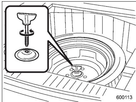
6. Turn the attaching bolt counterclockwise, then take spare tire out.
