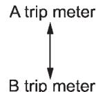
To set the trip meter to zero, select the A trip or B trip meter by pushing the knob and keep the knob pushed for more than 2 seconds.
