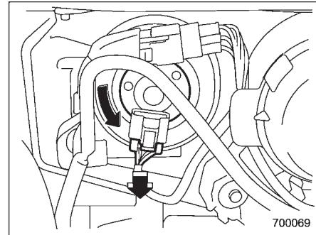
3. Disconnect the electrical connector from the bulb.
