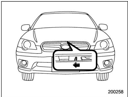
3. Release the secondary hood release located under the front grille by moving the lever toward the left.
