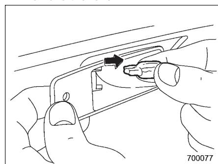
3. Pull the bulb out of the socket. Install a
