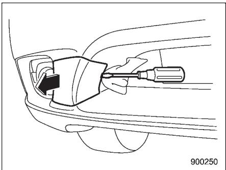
4. Likewise, insert the screwdriver still wrapped with cloth or vinyl into the cutout between the towing hook cover and the bumper. Pry out the cover.
