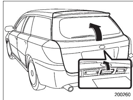
The rear gate can be locked and unlocked using either the keyless entry system or the power door locking switch.
