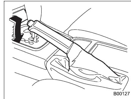
Check the parking brake stroke according to the maintenance schedule in the "Warranty and Maintenance Booklet". When the parking brake is properly adjusted, braking power is fully applied by pulling the lever up five to six notches gently but firmly (approximately 44 lbs, 196 N, 20 kg). If the parking brake lever stroke is not within the specified range, have the brake system checked and adjusted at your SUBARU dealer.
