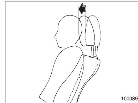
The front seats of your vehicle are equipped with active head restraints. They automatically tilt forward slightly in the
