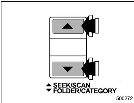
The scan mode lets you listen to the first 10 seconds of each track/file (track) in succession. Press the “▲” side of the SEEK/SCAN button for 0.5 second or longer to start scanning upward beginning with the track/file (track) following the currently selected one. Press the “▼” side of the button to start scanning downward beginning with the track/file (track) preceding the currently selected one.
