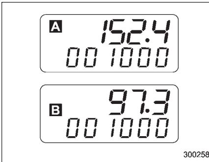
This meter displays the two trip meters when the ignition switch is in the "LOCK", "ACC" or "ON" position.
