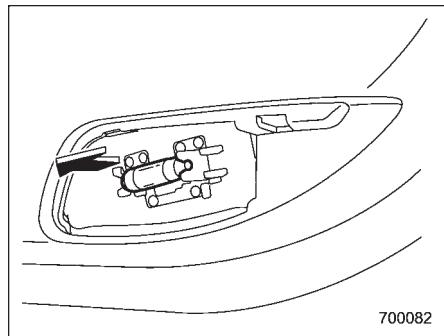
2. Pull the bulb out of the socket. Install a new bulb.
