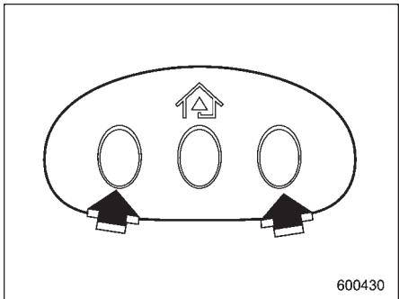
2. Press and hold the two outside HomeLink® buttons until the indicator light begins to flash (after 20 seconds). Release both buttons.
