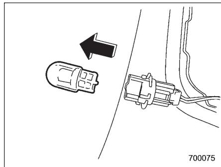
3. Pull the bulb out of the bulb socket and replace it with a new one.
