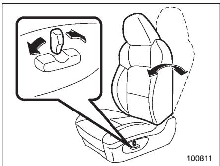
To adjust the angle of the seatback, move the control switch.
