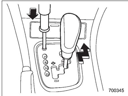
If you inadvertently have turned the ignition switch to the "OFF" position with the selector lever in the "N" position, proceed as follows. By referring to the "Shift lock release" section in this chapter, remove the shift lock release cover. Then, with the screwdriver inserted into the hole, move the selector lever to the "P" position. If the selector lever reverse inhibiting function fails, have the vehicle inspected by the
