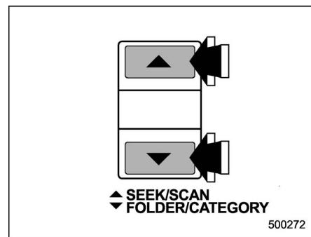
If you press the "▲" or "▼" side of the SEEK/SCAN button for 0.5 second or longer, the radio will switch to scan mode. In this mode, the radio scans through the radio band until a station is found. The radio will stop at the station for five seconds while displaying the frequency, after which scanning will continue until the entire band has been scanned.
