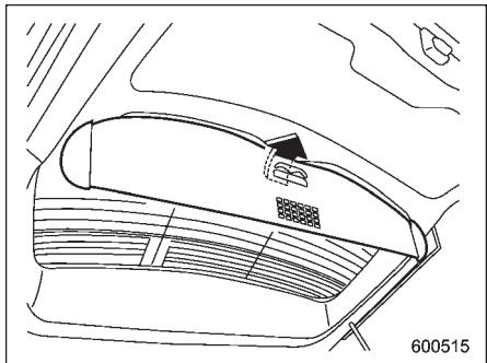
Rotate the rear gate board toward you until its top touches the rear gate panel.
