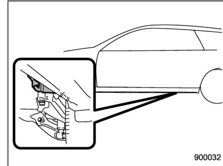
The rear tie-down hooks are located near each of the jack-up reinforcements.
