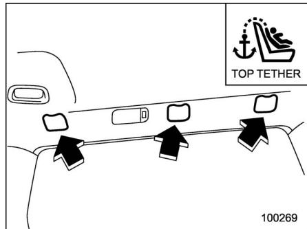
Three tether anchorages, i.e., ones for the right, center and left positions, are already installed on the rear edge of the roof. Open the cover flap to use each anchorage.
