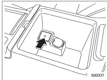
By connecting a commercial audio product to the vehicle, such as portable audio player, you can hear its sound via the vehicle's speaker.
