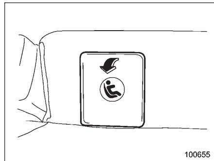
Remove the two covers from the selected side of the rear seatback to expose the anchorages (bars) to be used for installation of the child restraint system.
