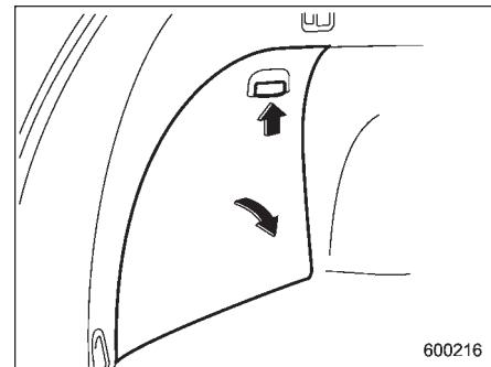
A stowage box is located on each side of the cargo area. You can access each one by pushing up and pulling the knob on the lid.
