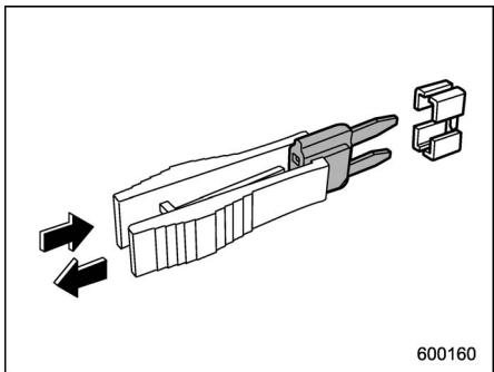
4. Pull out the fuse with the fuse puller.
