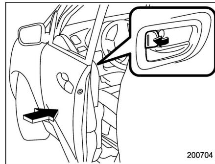
4. Before closing the doors, lock all doors with the inside door lock levers.
