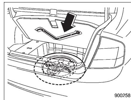
**Sedan:** Open the floor cover and remove the jack handle from the back of the floor cover.
