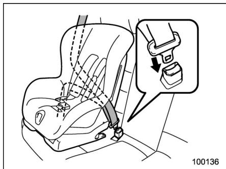
1. Place the child restraint system in the seating position.
