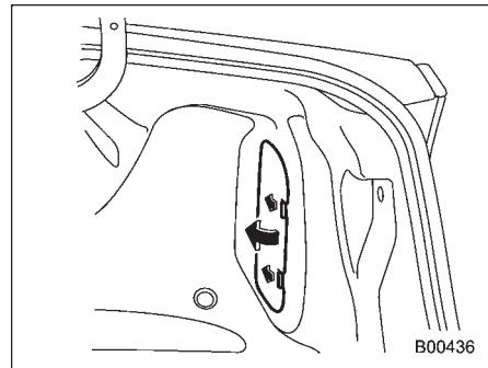
1. Push the knobs of the cover to open the cover.
