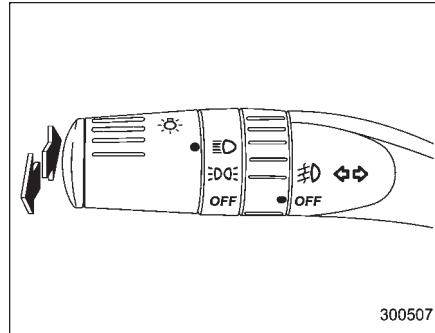
To change from low beam to high beam, push the turn signal lever forward. When the headlights are on high beam, the high beam indicator light " $\odot\odot$ " on the instrument panel is also on.
