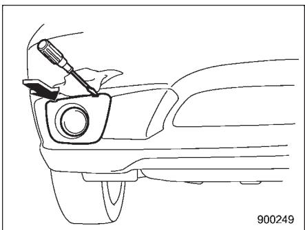
2. Wrap a flat-head screwdriver with cloth or vinyl. Then, insert the screwdriver into the gap between the front fog light cover and the bumper, and pry out the cover.
