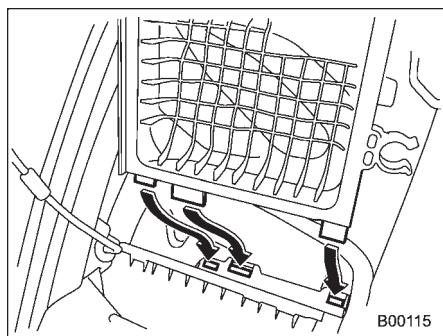
7. To install the air cleaner case cover, insert the three projections on the air cleaner case cover into the slits on the air cleaner case and then snap the two clamps on the air cleaner case cover.
