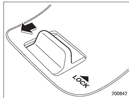
6. When you have finished entering the number, pull the lock knob to the "UN-LOCK" side within five seconds.
