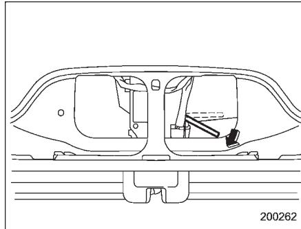
3. Unlock the rear gate by pressing the lever inside the trim downward.
