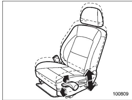
The height of the seat can be adjusted by moving the seat cushion adjustment lever up and down.
