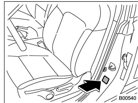
Check the tire pressures when the tires are cold. Use a pressure gauge to adjust the tire pressures to the values shown on the tire placard. The tire placard is located on the door pillar on the driver's side.
