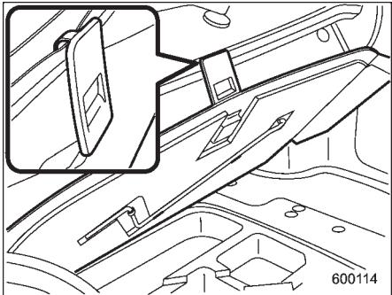
1. Lift the handle of the floor cover and hook the handle onto the trunk edge.
