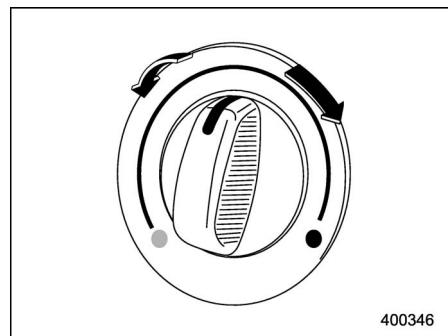
This dial regulates the temperature of air flow from the air outlets over a range from the blue side (cool) to red side (warm).
