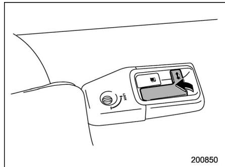
Pull the trunk lid release lever upward.
