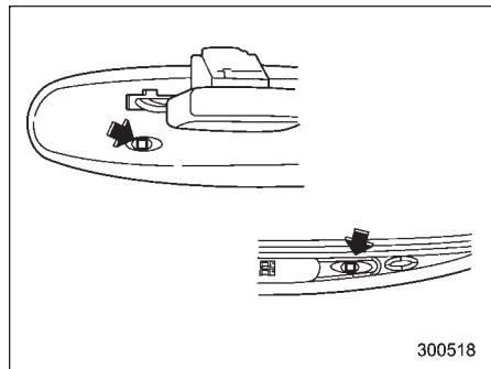
The mirror has a photosensor attached on both the front and back sides. If the glare from the headlights of vehicles behind you strikes the mirror, these sensors detect it and make the reflection surface of the mirror dimmer to help prevent you from being blinded. For this reason, use care not to cover the sensors with stickers, or
