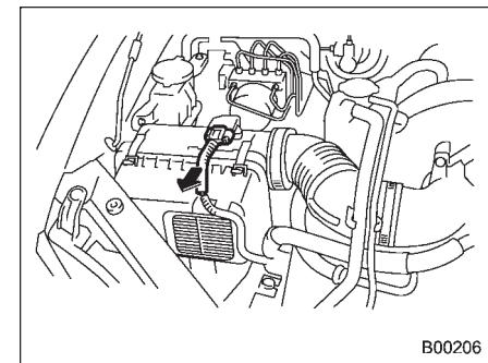
2. Unplug the connector that is attached to the top of the air cleaner case.
