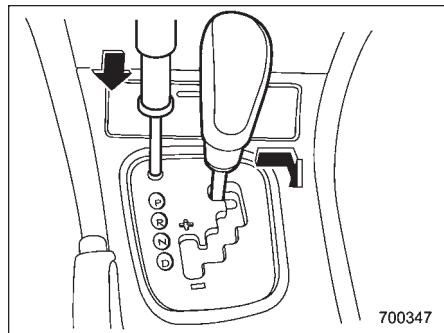
4. Insert the screwdriver into the hole.
