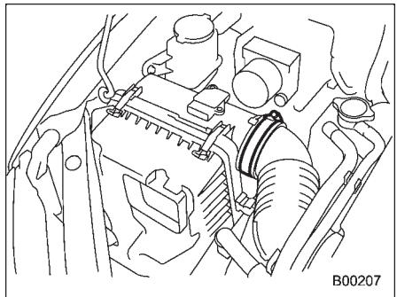
3. Use a screwdriver to remove the duct that is connected to the air cleaner case cover.
