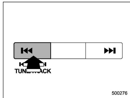
Briefly press the "◀" side of the TUNE/TRACK button to skip to the beginning of the current track/file (track). Each time the button is pressed, the indicated track/file (track) number will decrease.
