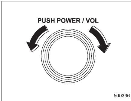
The volume control dial normally functions as a volume control. This dial becomes a control for Bass, Midrange, Treble, Fader or Balance when you select the appropriate tone and balance control mode.
