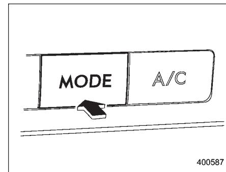
Select the desired air flow mode by pushing the air flow mode selection button. The selected air flow mode is shown by the display.
