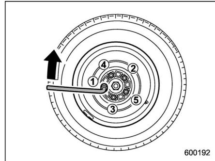
14. Use the wheel nut wrench to securely tighten the wheel nuts to the specified torque, following the tightening order in the illustration.
