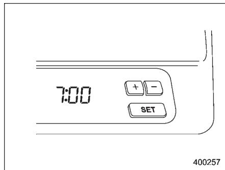
The clock shows the time while the ignition switch is in the “ACC” or “ON” position.
