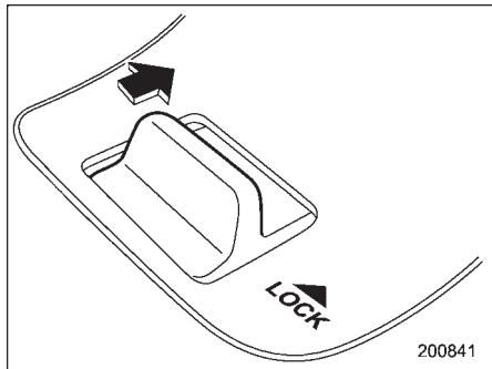
5. Before the electronic tone stops sounding, press the power door lock knob to the "LOCK" side the same number of times as the leftmost digit of the transmitter code. For example, press the lock knob eight times if the leftmost digit of the code is 8.
