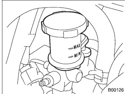
Check the fluid level on the outside of the reservoir. If the level is below "MIN" level mark, add the recommended clutch fluid to "MAX" level mark.
