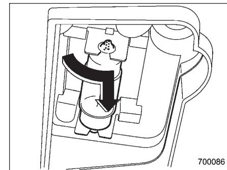
2. Turn the bulb until the flat surfaces at its ends are aligned vertically. Pull the bulb
