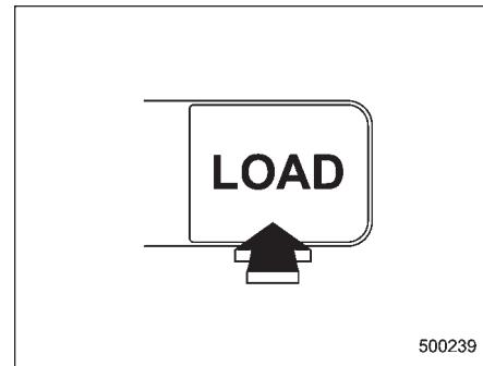
1. If you continue to press the "LOAD" button for more than 1.5 seconds, the player will produce beep sound and will enter the full disc loading mode.
