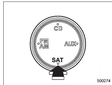
Push the "SAT" button when the radio is off to turn on the radio.
