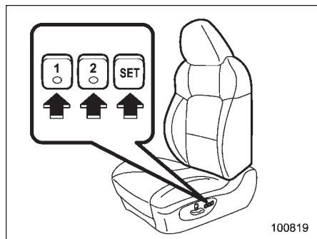
3. While pressing the "SET" button, press the desired button "1" or "2".
