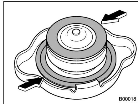
7. Put the radiator cap back on and tighten firmly. At this time, make sure that
