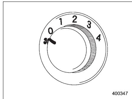
The fan operates only when the ignition switch is turned to the "ON" position. The fan speed control dial is used to select four fan speeds.
