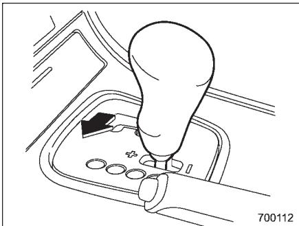
SPORT mode is used when power is needed for rapid acceleration or for uphill driving. To select this mode, move the selector lever from the "D" position to the manual gate.
