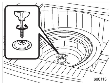
6. Turn the attaching bolt counterclockwise, then take the spare tire out.
