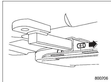
2. Insert the hitch pin into the hole on the hitch receiver tube so that the pin passes through the ball mount.
