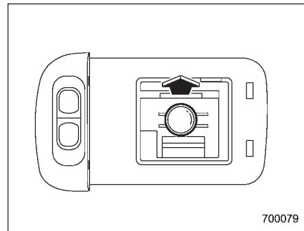
3. Pull the bulb out of the socket. Install a new bulb.
