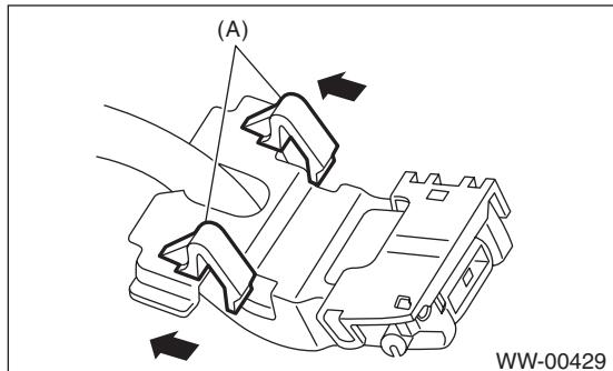
3) Remove the washer hose from the washer nozzle.
