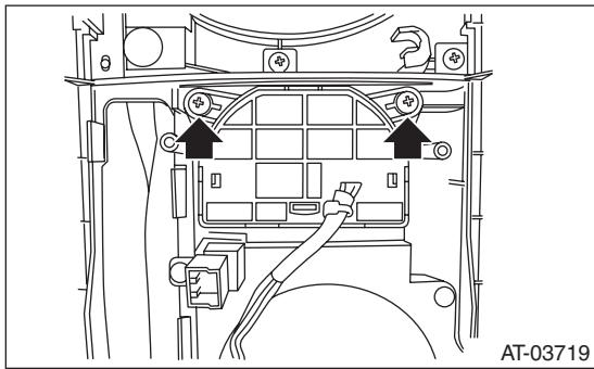
5) Remove the screws which secure the cup holder to the console box, then remove the SI-DRIVE selector.
