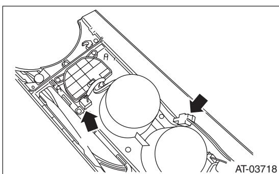
4) Remove the screws securing the upper side of the SI-DRIVE selector to the console box.
