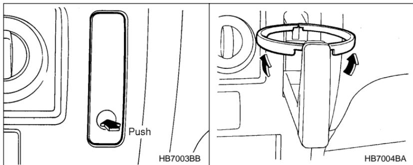
The cup holder is located beside the climate control panel. To use the cup holder, push on its front surface and it will automatically pop out. Then pull it out completely.
