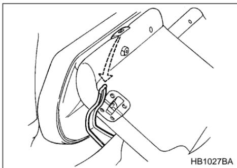
7. Install the headrest (if so equipped) onto the backside of the seatback.
