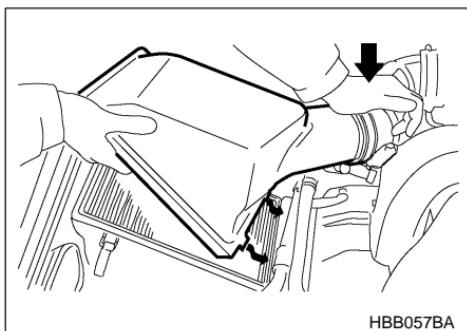
To install the air cleaner case cover, insert two projections on the air cleaner case into the slits on the air cleaner case cover and then snap the two clamps on the air cleaner case cover.
