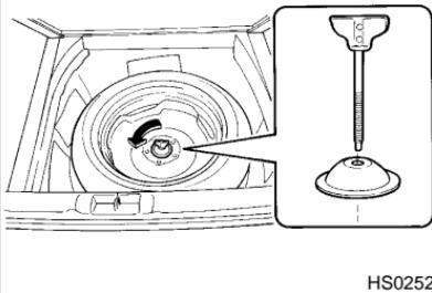
The spare tire is stored under the floor of the trunk or cargo area.
