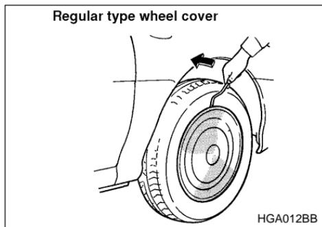
Insert the wheel nut wrench into the notch provided, and pry the wheel cover off.
