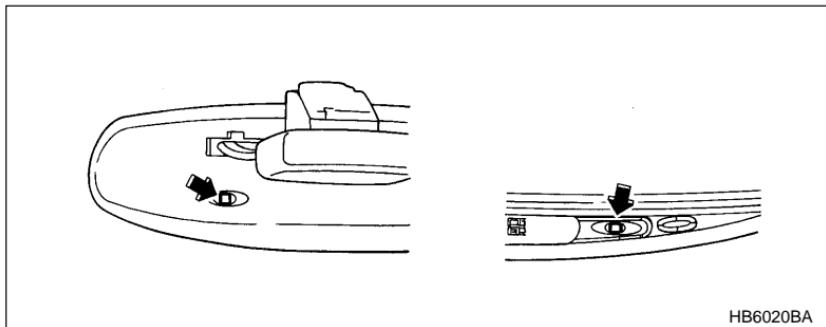
The mirror has a photosensor attached on both the front and back sides. If the glare from the headlights of vehicles behind you strikes the mirror, these sensors detect it and make the reflection surface of the mirror dimmer to help prevent you from being blinded. For this reason, use care not to cover the sensors with stickers, or other similar items. Periodically wipe the sensors clean using a piece of dry soft cotton cloth or an applicator.
