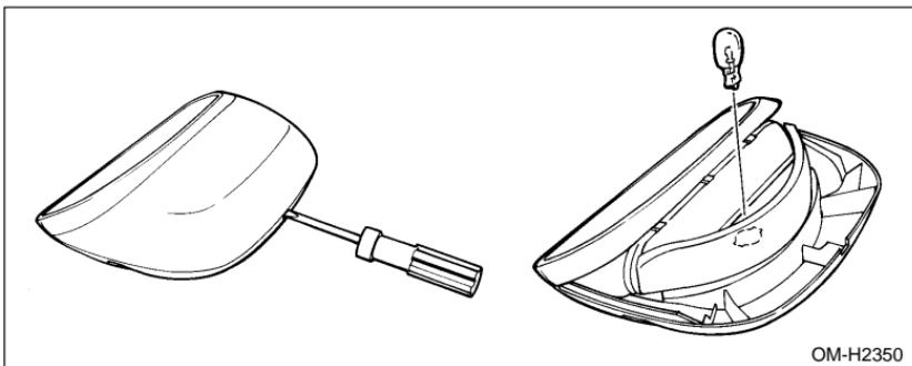
1. Remove the high mount stop light cover by prying on the edge with a screwdriver.
