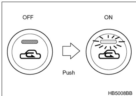
**ON position:** Interior air is recirculated inside the vehicle. Push the air inlet selection button to the ON position. The indicator light will come on.
