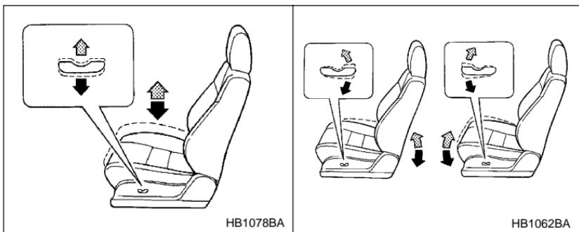
To adjust the angle and height of the seat cushion, move the control switch in the corresponding direction.
