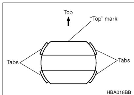
**When installing the protector, make sure the "TOP" mark is at the top.**
