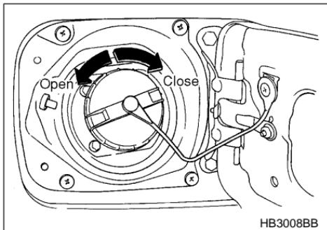
2. Remove the fuel filler cap by turning it slowly counterclockwise.
