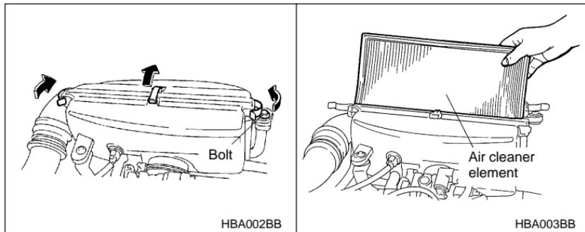
1. Remove the bolt securing the rear air cleaner element case.
