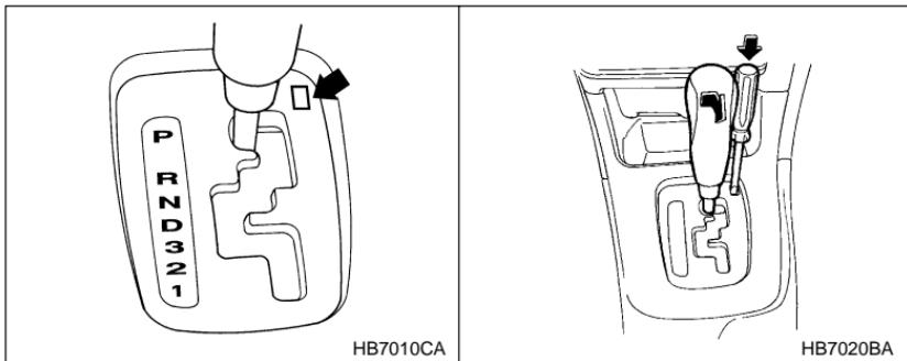
4. Insert the screwdriver into the hole.
