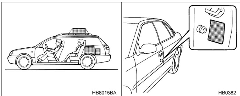
The load capacity of your vehicle is determined by weight, not by available cargo space. The maximum load you can carry in your vehicle is shown as the Vehicle Capacity Weight on the tire information label attached to the driver's side door jamb. It includes the total weight of driver and all passengers and their belongings, any optional equipment such as a trailer hitch, roof rack or bike carrier, etc., and the tongue load of a trailer.
