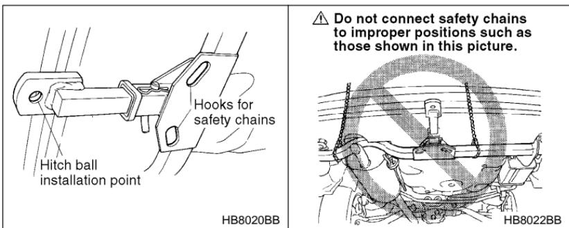
**⚠ Do not connect safety chains to improper positions such as those shown in this picture.**
