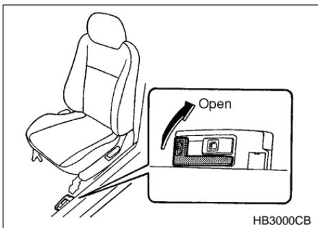
Pull the trunk lid release lever upward.
