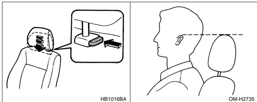
To raise the head restraint, pull it up. To lower it, push the head restraint down while pressing the release button on the top of the seatback.
