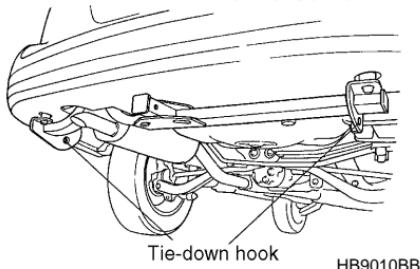
The towing hooks should be used only in an emergency (e.g., to free a stuck vehicle from mud, sand or snow).
