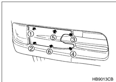
2. Push the towing hook cover in accordance with the pushing order given in the illustration.
