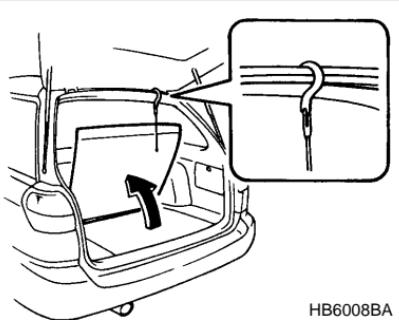
The storage tray is located under the floor of the trunk or cargo area and can be used to store small items. To open the lid, pull the tab or handle up.
