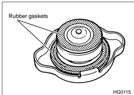
5. Put the radiator cap back on and tighten firmly. At this time, make sure that the rubber gasket in the radiator cap is correctly in place.
