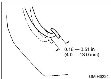
Lightly press the clutch pedal down with your finger until you feel resistance, and check the free play.
