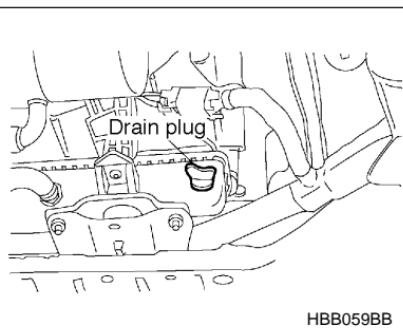
3. Loosen the radiator cap to drain the coolant from the radiator. Then drain the coolant from the reserve tank. Tighten the drain plug securely.
