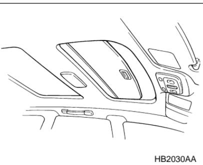
The front moonroof has a tilting function and the rear moonroof has a sliding function.
