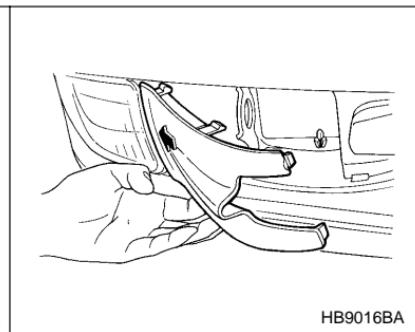
1. Insert the towing hook cover into the clearance between the fog light (or bumper trim cover) and the bumper body.
