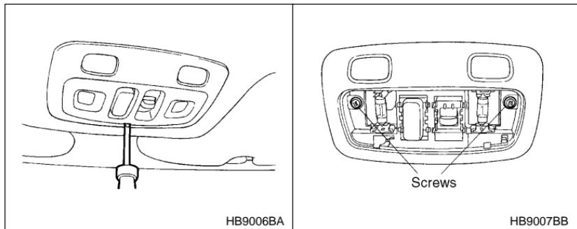
2. Remove the spot light lens by prying the edge of the lens with a regular screwdriver, then remove the switch body retaining screws and take off the moonroof switch.
