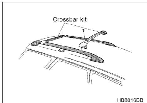
The roof rail is not designed to carry cargo by itself. Cargo can be carried after securing the roof crossbar kit to the roof rail and installing the appropriate carrying attachment. When installing the roof crossbar kit, follow the manufacturer's instructions.
