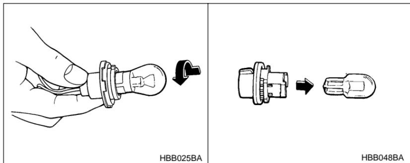
5. Remove the bulb from the socket.
