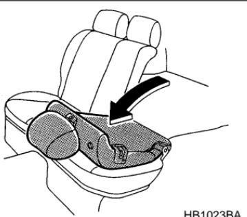
Unlock the seatback by pulling the release knob and then fold the seatback down.
