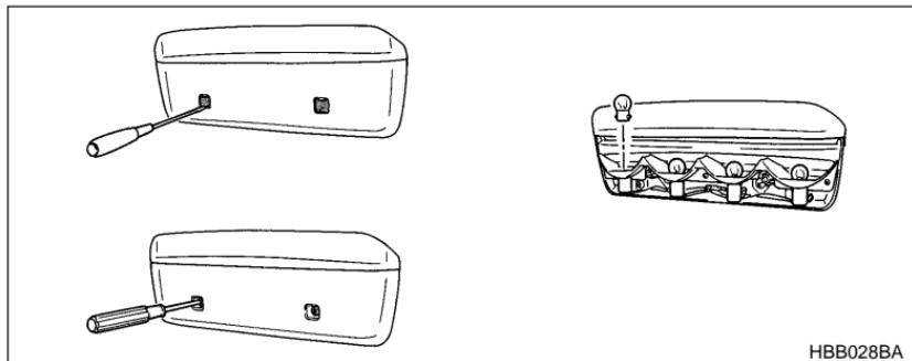
1. Remove the mounting screw covers by prying on the edge with a screwdriver.
