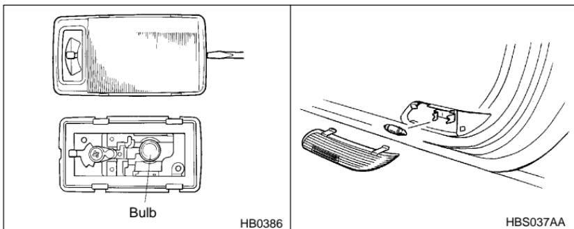
1. Remove the lens by prying the edge of the lens with a regular screwdriver.
