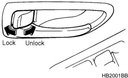
To lock the door from the inside, rotate the lock lever rearward. To unlock the door from the inside, rotate the lock lever forward.
