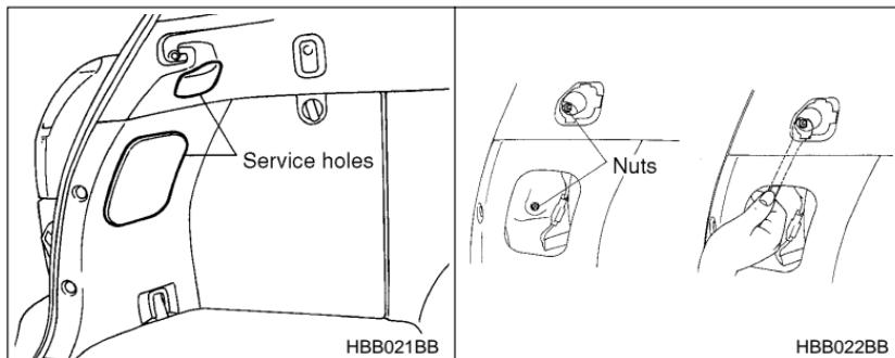
1. Remove the light bulb replacement service hole covers at two places by prying the edge of the cover with a regular screwdriver.
