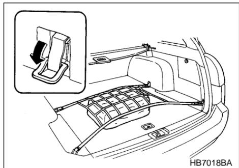
The cargo area is equipped with four anchorage eyelets so that cargo can be secured with a luggage net or ropes.
