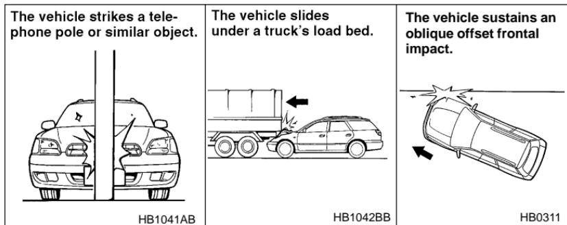
▽ **Examples of the types of accidents in which the SRS frontal airbag will basically not deploy.**
