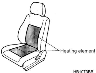
To turn on the seat heater, push the "LO" or "HI" position on the switch, as desired, depending on the temperature.
