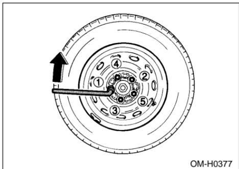
The torque for tightening the nuts is 58 to 72 ft-lb (78 to 98 N-m, 8 to 10 kg-m). This torque is equivalent to applying about 88 to 110 lbs (40 to 50 kg) at the top of the wheel nut wrench. Never use your foot on the wheel nut wrench or a pipe extension on the wrench because you may exceed the specified torque. Have the wheel nut torque checked at the nearest automotive service facility.
