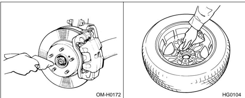
12. Put on the spare tire. Replace the wheel nuts. Tighten them by hand.
