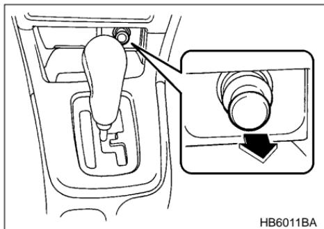
The electrical power socket located on the lower part of the instrument panel can only be used as cigarette lighter socket. A cigarette lighter plug is an optional accessory. It is available from your SUBARU dealer. If smoking is not desired, always put the cap on the socket to prevent any foreign object from entering it.
