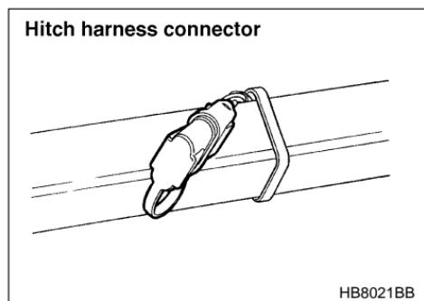
9. Confirm proper function of the hitch wire harness by individually activating the brake, right turn signal, left turn signal, stop, and parking lights on the trailer.
