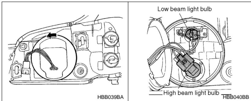
Remove the headlight bulb cover, by turning it counterclockwise.
