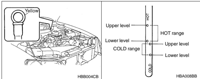
4. Pull out the dipstick and check the fluid level on the gauge. If it is below the lower level on the "HOT" range, add the recommended automatic transmission fluid up to the upper level.
