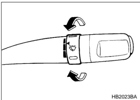
When the wiper switch is in the "OFF" position, turn the dial to adjust the operating interval of the wiper.
