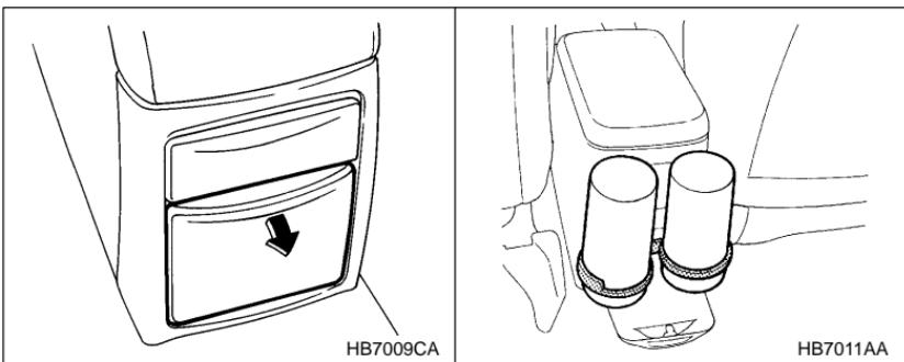
The rear passenger's cup holder is located on the lower side of the back of the center console. To use the cup holder, open the lid by pulling its upper edge.
