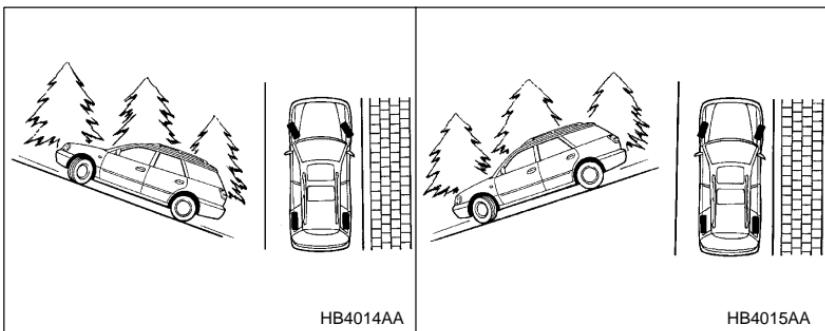
When parking on a hill, always turn the steering wheel. When the vehicle is headed up the hill, the front wheels should be turned away from the curb. When facing downhill, the front wheels should be turned into the curb.
