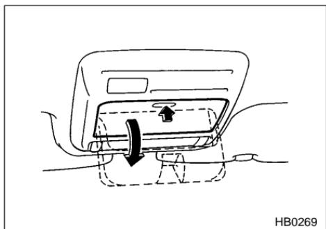
To open the console, push on the lid lightly and it will automatically open.
