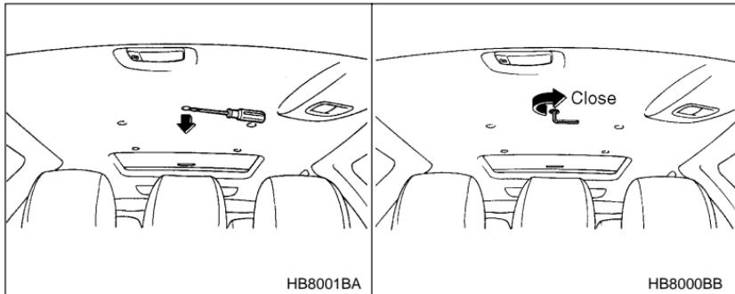
2. Remove the plug on the roof trim by inserting the end of the regular screwdriver between the roof and plug and prying it off.
