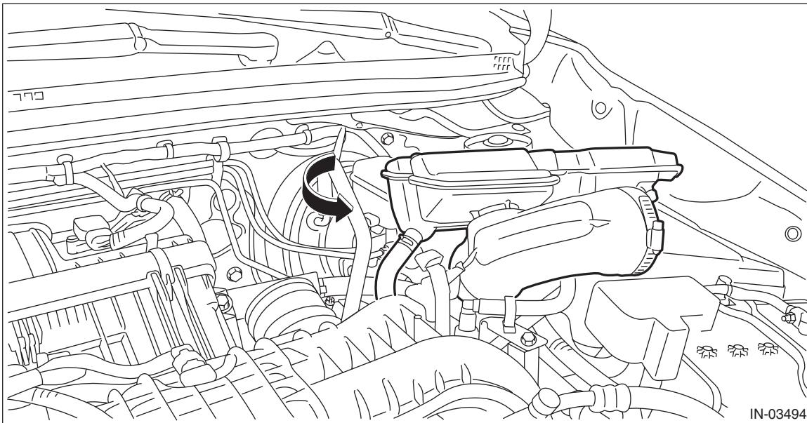
5) Remove the air intake boot No. 2 from the throttle body.
