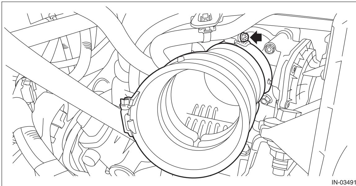
2) Install the resonator chamber. <Ref. to IN(H4DO(HEV))-19, INSTALLATION, Resonator Chamber.>
