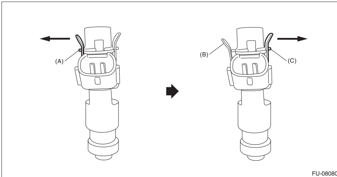
(3) Remove the fuel injector holder from the fuel pipe and fuel injector, and remove the fuel injector from the fuel pipe.
