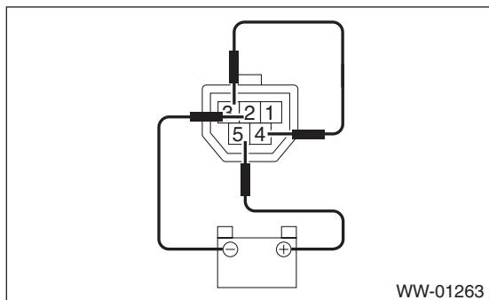
(3) Connect the battery to terminals of the connector, and remove the terminal connection with motor rotating at low speed, and stop the motor assembly - windshield wiper in mid-operation.
