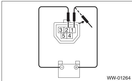
(4) Connect the battery and check that the motor stops at the automatic stop position after the motor operates at low speed again.
