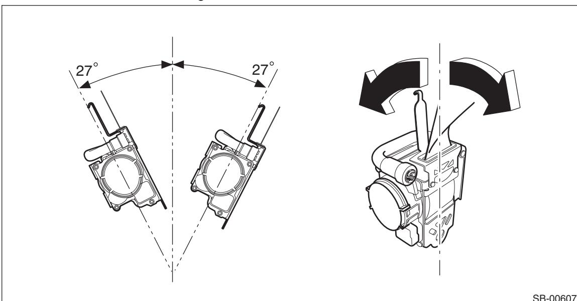
3) If the ELR lock mechanism does not operate properly, replace the seat belt outer - front with a new part.
