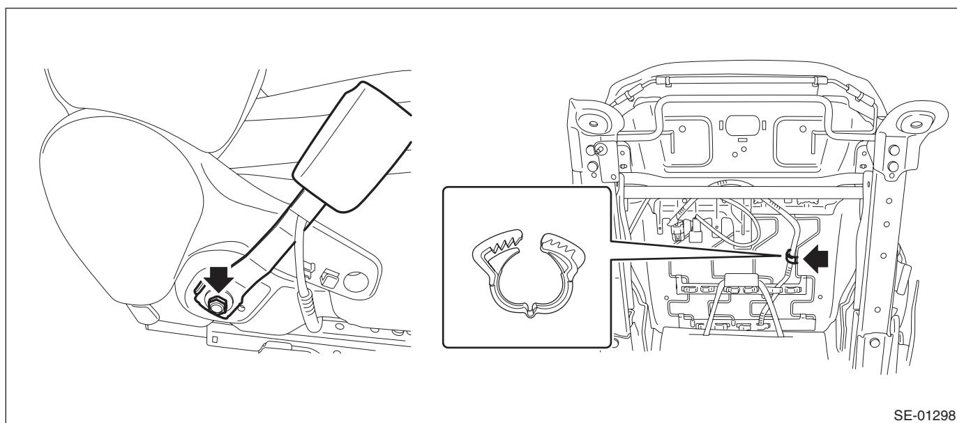
3) Install the seat assembly to the body.
