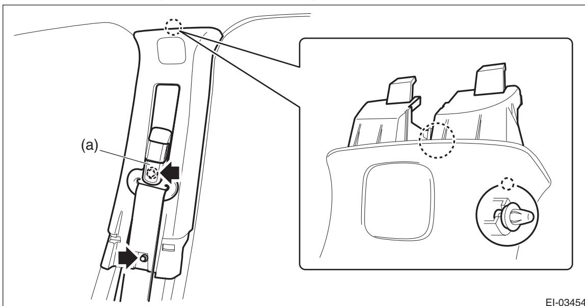
8) Remove the bolts, and then remove the adjuster assembly - seat belt.
