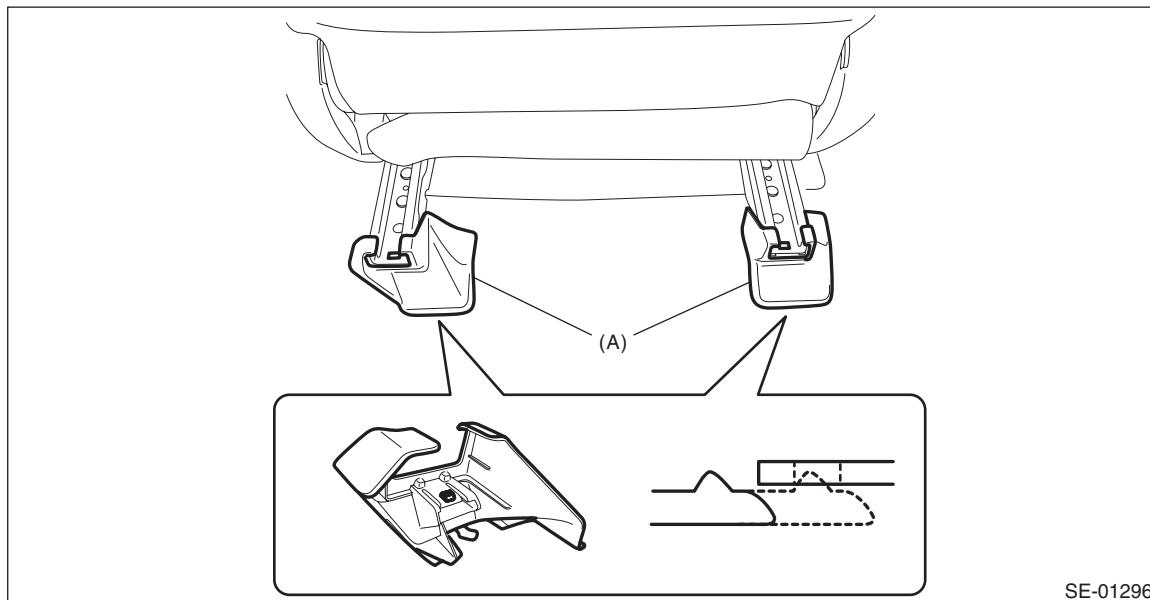
(3) Move the front seat to the rearmost position, and remove the bolts.
