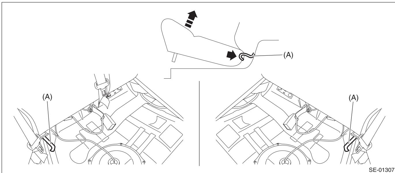
5) Release the clips and claws, and then remove the cover side sill - rear INN.
