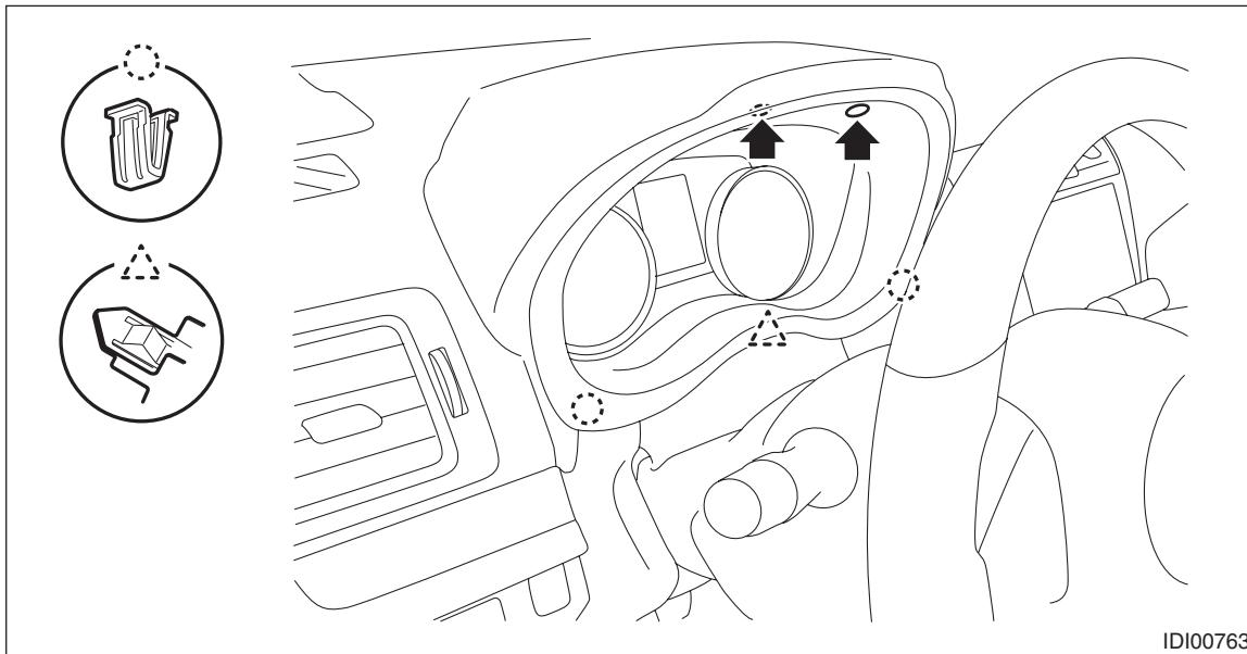
4) Remove the combination meter assembly.
