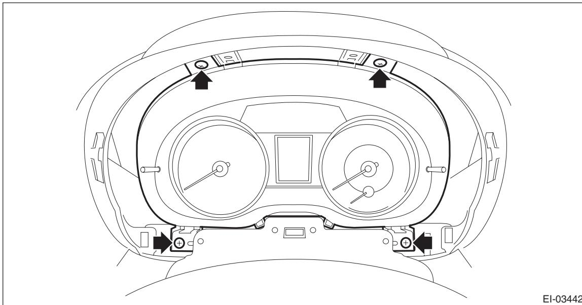
(2) Pull the combination meter assembly toward you and disconnect the connector.
