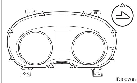
2) Release the claws, and then remove the visor - combination meter.
