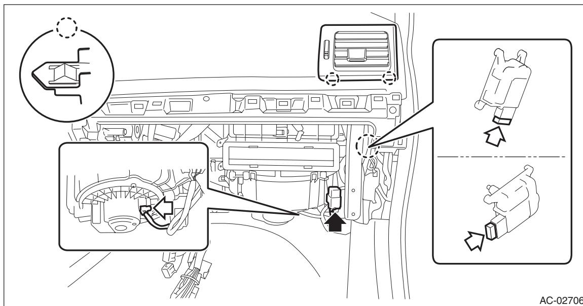
(3) Remove the bolts and nuts to remove blower motor unit assembly.
