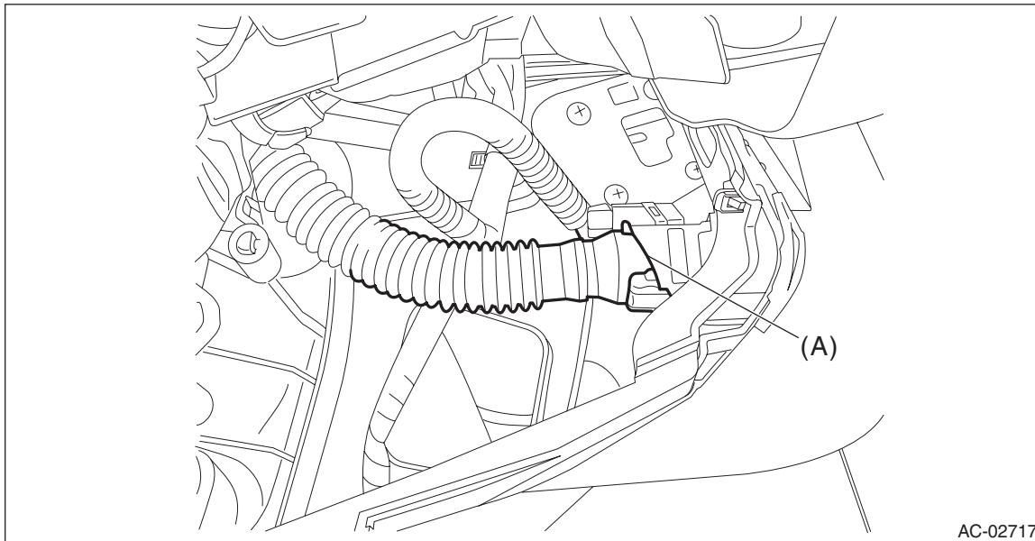
(1) Are the aspirator hoses on both sides of the case and sensor connected securely?
