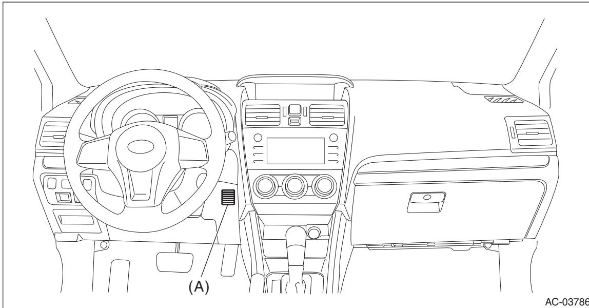
(1) Put a strip of paper close to the front side of the suction port (A).
