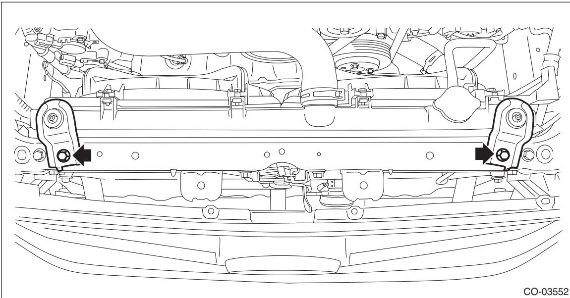
6) Remove the condenser assembly - air conditioner.
