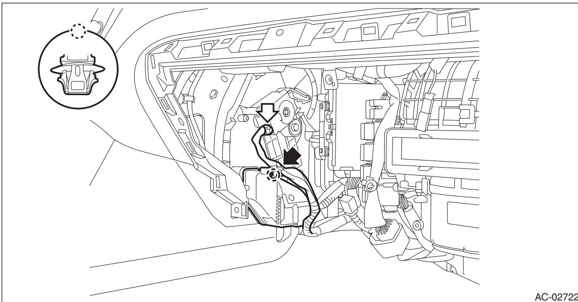
4) Remove the power transistor.
