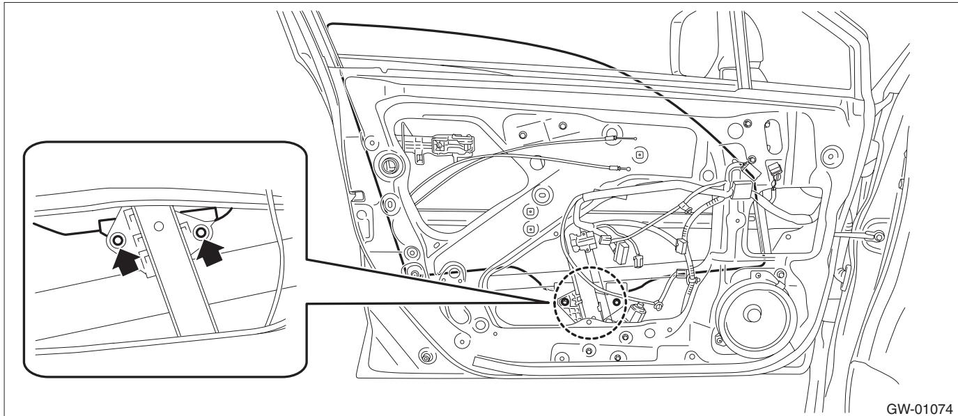
(4) While tilting the glass, remove the glass assembly - front door.
