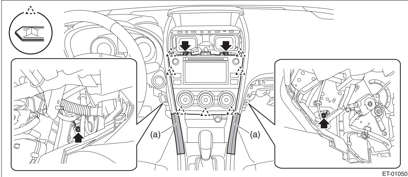
6) Remove the screws, and then remove the audio bracket.
