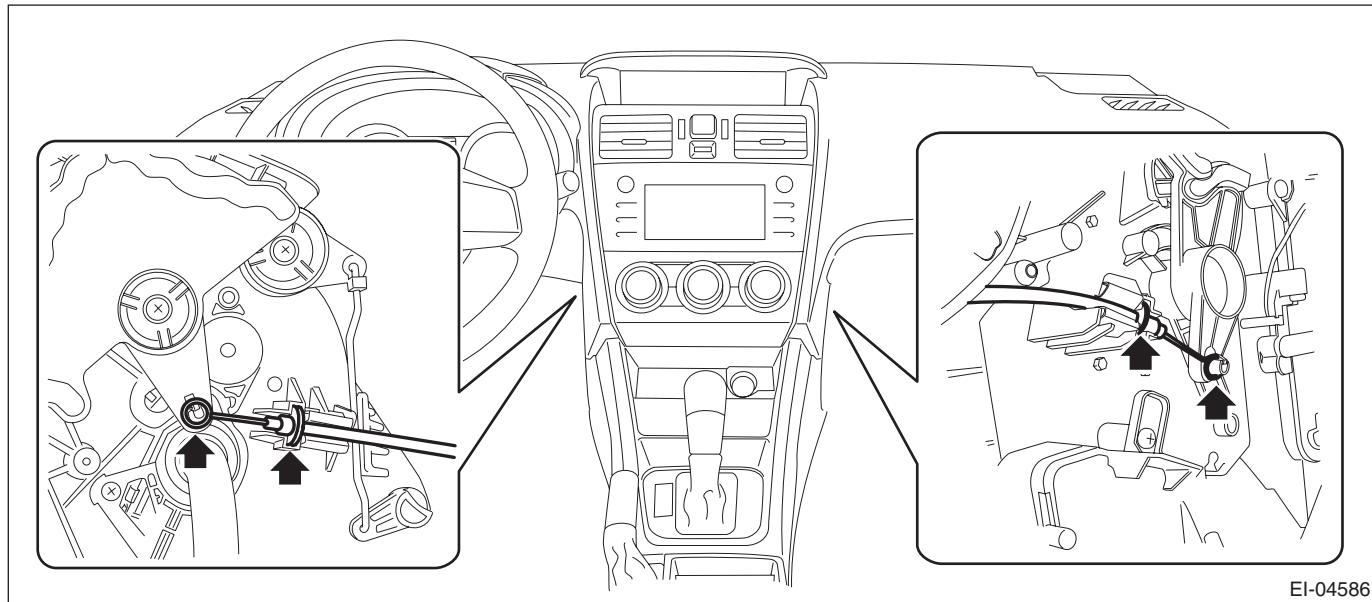
(2) Attach the protective tape (a) to the cover - shift lever.
