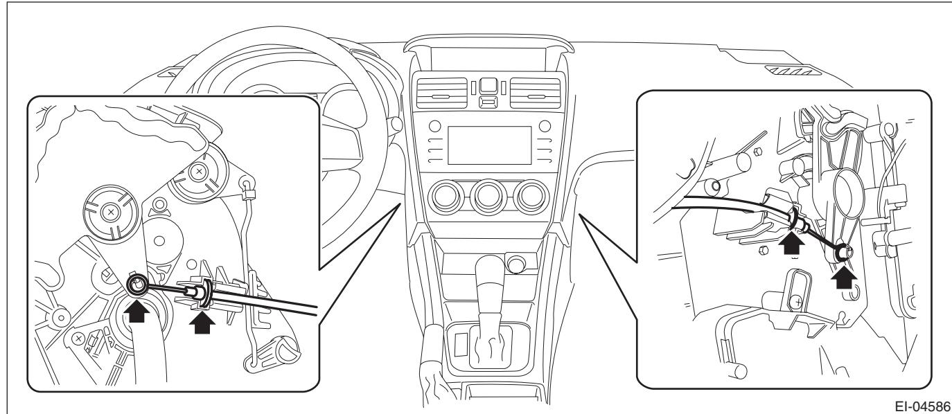
6) Remove the center grille assembly. <Ref. to AC-104, REMOVAL, Air Vent Grille.>
