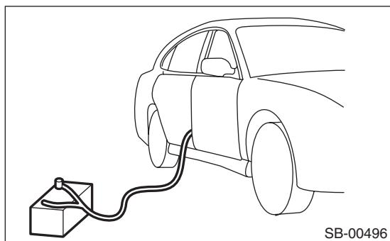
10) Move the battery at least 5 m (16 ft) from the vehicle, and confirm safety in the area.
