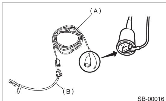
7) Connect test harness adapter AM to airbag connector.
