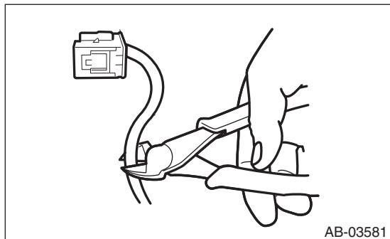
6) Peel off the shield approx. 20 mm (0.79 in) from the two harnesses of the removed body side connector.
