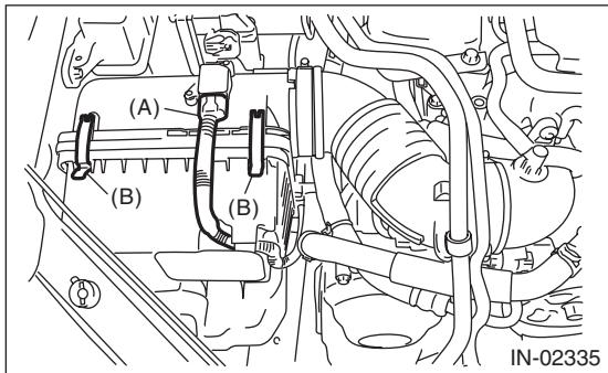
5) Open the air cleaner case, and remove the air cleaner element.
