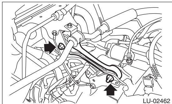
25) Attach ST to the fuel delivery pipe and push ST in the direction of arrow mark to disconnect the fuel delivery hose.
