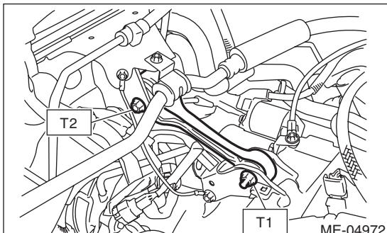
8) Install the starter. <Ref. to SC(STI)-8, INSTALLATION, Starter.>
