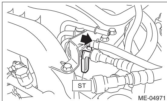
27) Remove the clip and disconnect the evaporation hose from the fuel pipe.
