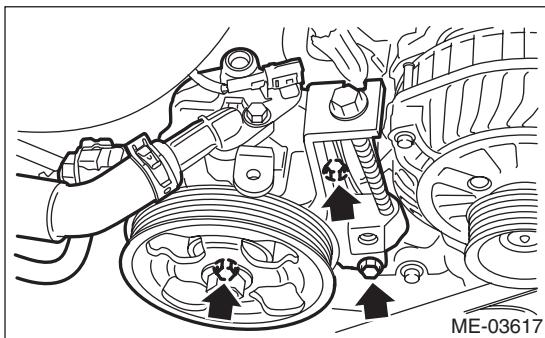
(2) Connect the connector to the power steering pump switch.
