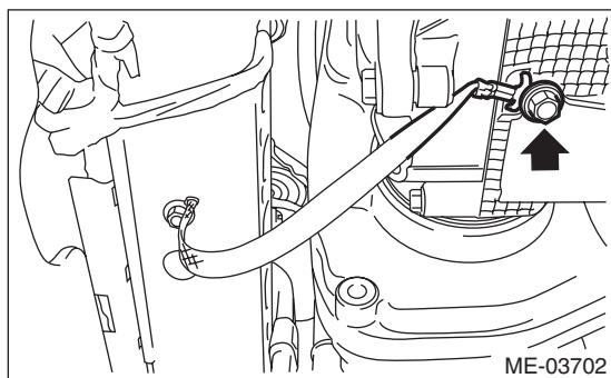
14) Install the joint pipe and front exhaust pipe.
