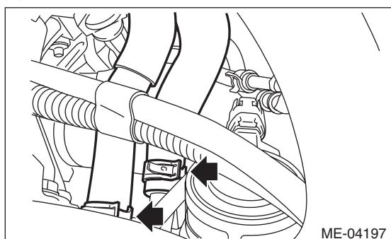
16) Remove the power steering pump.
