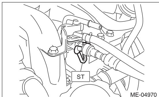
(3) Insert the back side of ST into the quick connector and push ST in the direction of arrow mark to disconnect the fuel return hose.
