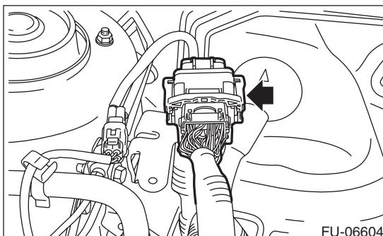
12) Remove the engine harness connector from the engine harness bracket.
