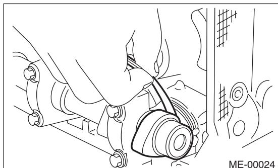
2) Remove the camshaft. <Ref. to ME(w/o STI)-59, REMOVAL, Camshaft.>
