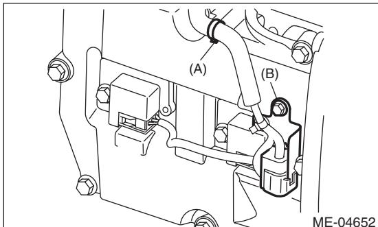
(2) Remove the ignition coil. <Ref. to IG(w/o STI)-8, REMOVAL, Ignition Coil.>
