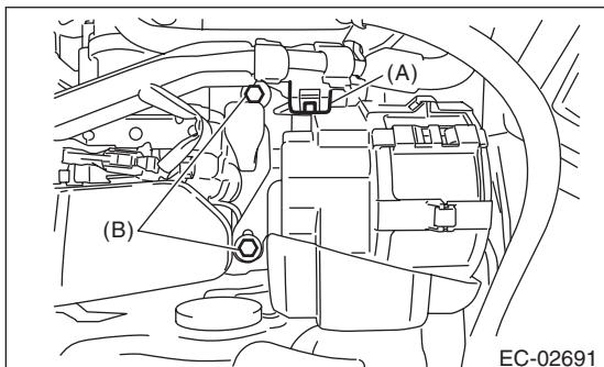
3) Disconnect the connector (A) and air duct (B) from secondary air pump and remove the secondary air pump.
