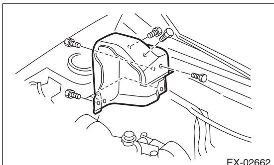
8) Remove the bolts which hold the upper side of the turbocharger lower cover.
