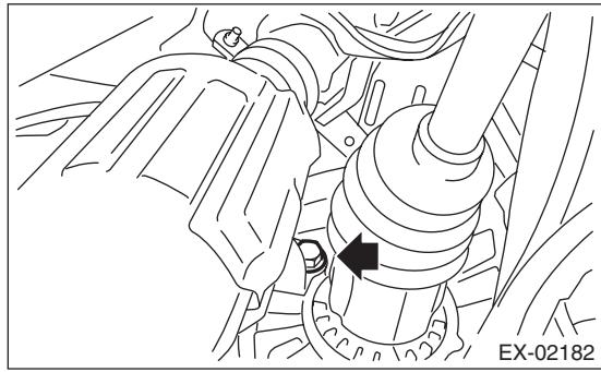
8) Tighten the bolts which secure the center exhaust pipe to the hanger bracket.
