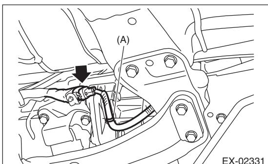
13) Remove the rear exhaust pipe from center exhaust pipe.
