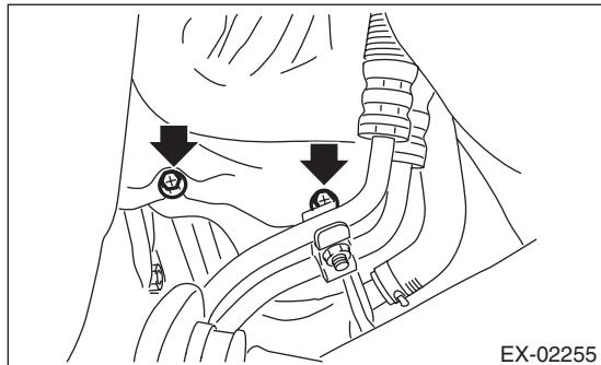
14) Install the transmission under cover. (6MT model)
