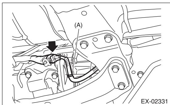
7) Tighten the bolt which holds center exhaust pipe to transmission.
