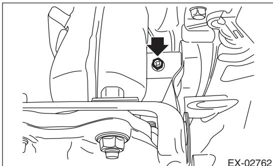
9) Remove the upper side bolts and nuts that hold the center exhaust pipe on the turbocharger, and remove the turbocharger cover stay (A).
