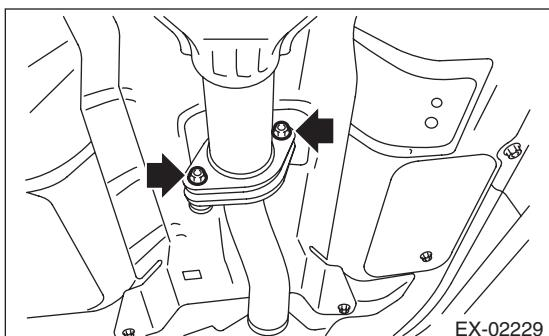
14) Remove the bolt which holds center exhaust pipe to transmission.
