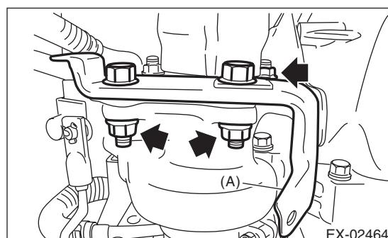
5) Install the rear exhaust pipe to center exhaust pipe.
