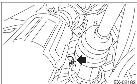
15) Remove the bolt which holds center exhaust pipe to hanger bracket, and remove the center exhaust pipe.
