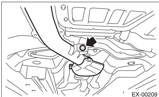
16) Remove the turbocharger lower cover.
