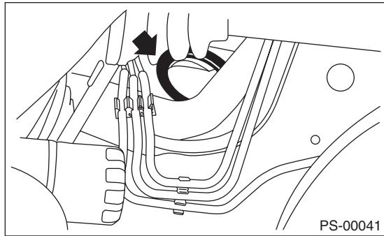
2) Insert the end of the steering shaft into the toe board grommet.
