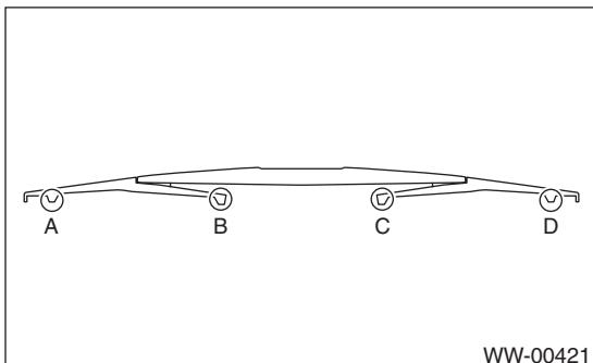
1) Insert the wiper rubber into claw (B).
