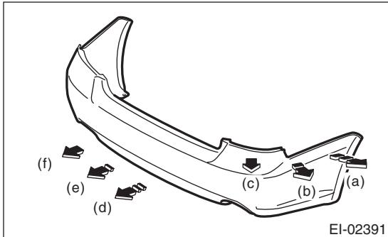
(1) Detach from the fender side in order from (a) to (c) while pulling up on the bumper face and twisting it towards you. (Both sides)
