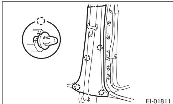
8) Spread the lower trim outwards to remove the claw, and pull on the upper trim to remove.
