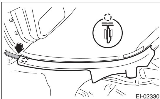
6) Remove weather strip (A) and door catcher cover (B), then remove the outside scuff plate.
